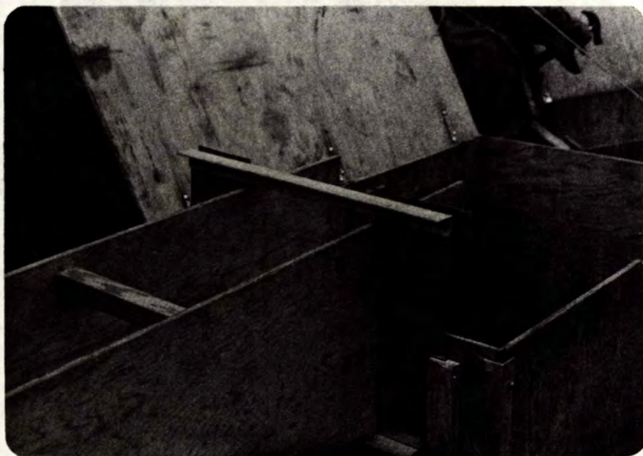
Plate 5. Adjustable trough flow regulator for downstream smolt transport into live box.
