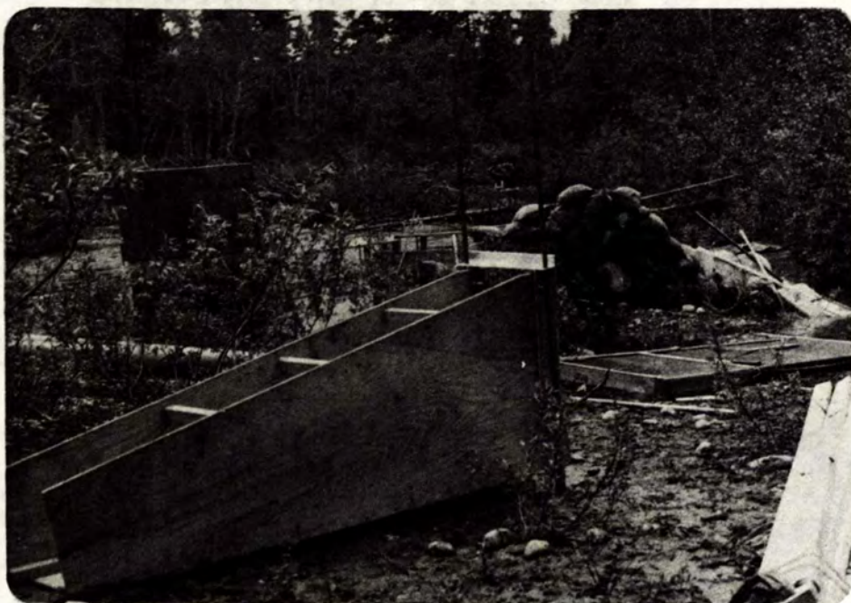
Plate 4. Modified hinge trough assembly for downstream "W" trap.
