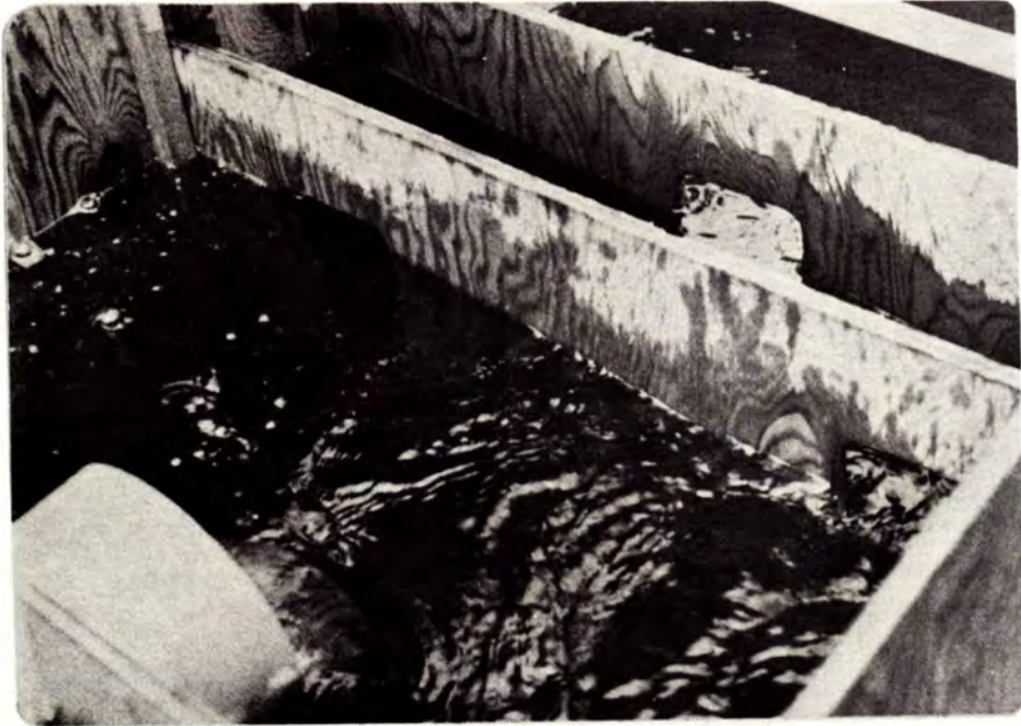
Plate 8: Interior of live box illustrating the staggered baffle arrangement which reduces turbulence and provides a sheltered holding region.
