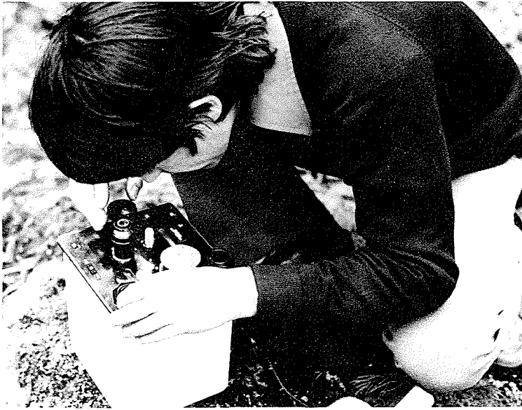
Reading a gravity meter at a field location.
