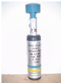
Signal Underwater Sound MK411 (Reduced Charge) (SUS) Signal Underwater Sound MK 410 (High Explosive)
