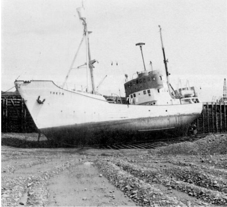
Plate 4. MV Theta resting on wooden "mattress" beside a jetty at low water. Parrsboro, Nova Scotia. (Photo by Canadian Hydrographic Service, 1960)
