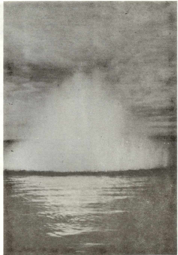
Photo 4. Surface dome caused by 10 lb of Geogel.
