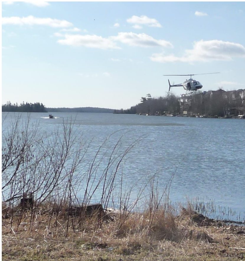
Figure 2b. Helicopter hovering to collect a water sample in Morris Lake by lowering the glug with a 2-L sampling bottle by rope to a depth of approximately 30-50 cm.
