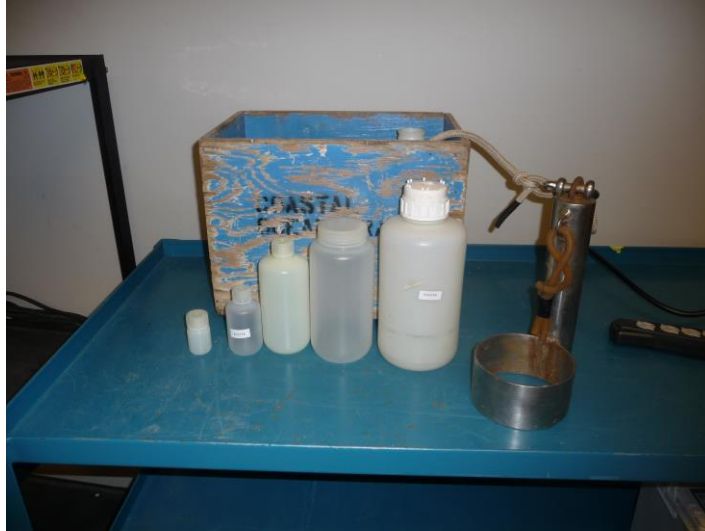
Figure 2a. Sampling gear. Right to left: weighted bottle holder (glug) attached to a rope, 2-L sampling bottle and subsampling bottles used in the lab.
