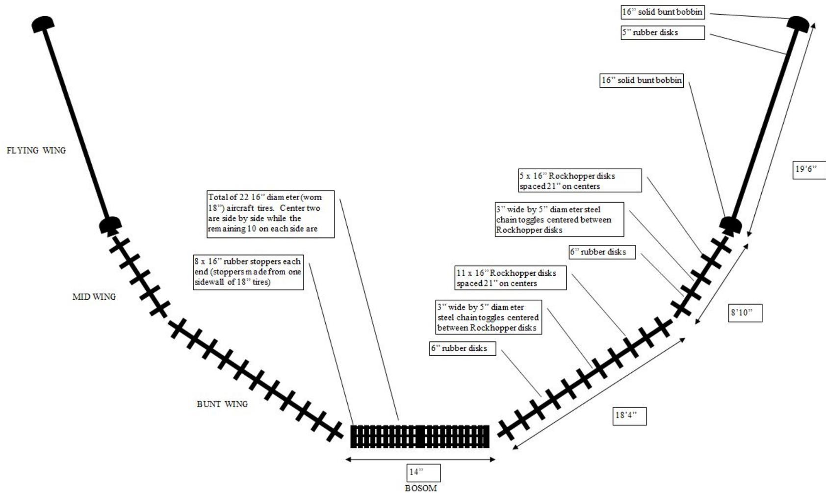
Figure 8. Details of the Rockhopper foot gear for the Atlantic Western Ila box trawl used on the 2016 WCVI synoptic bottom trawl survey.
