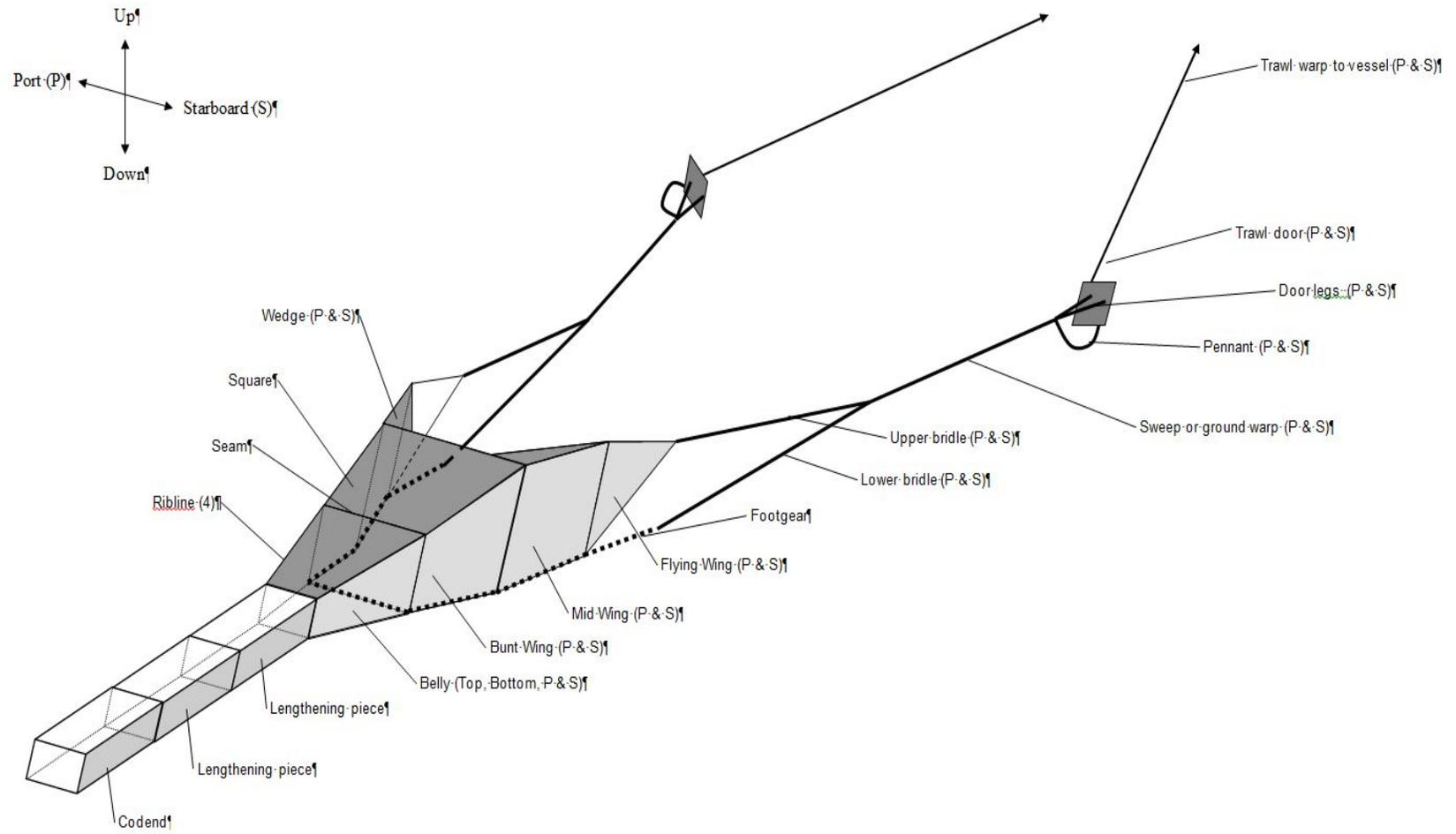
Figure 3. Overview diagram of the Atlantic Western IIA box trawl used on the 2016 WCVI synoptic bottom trawl survey.
