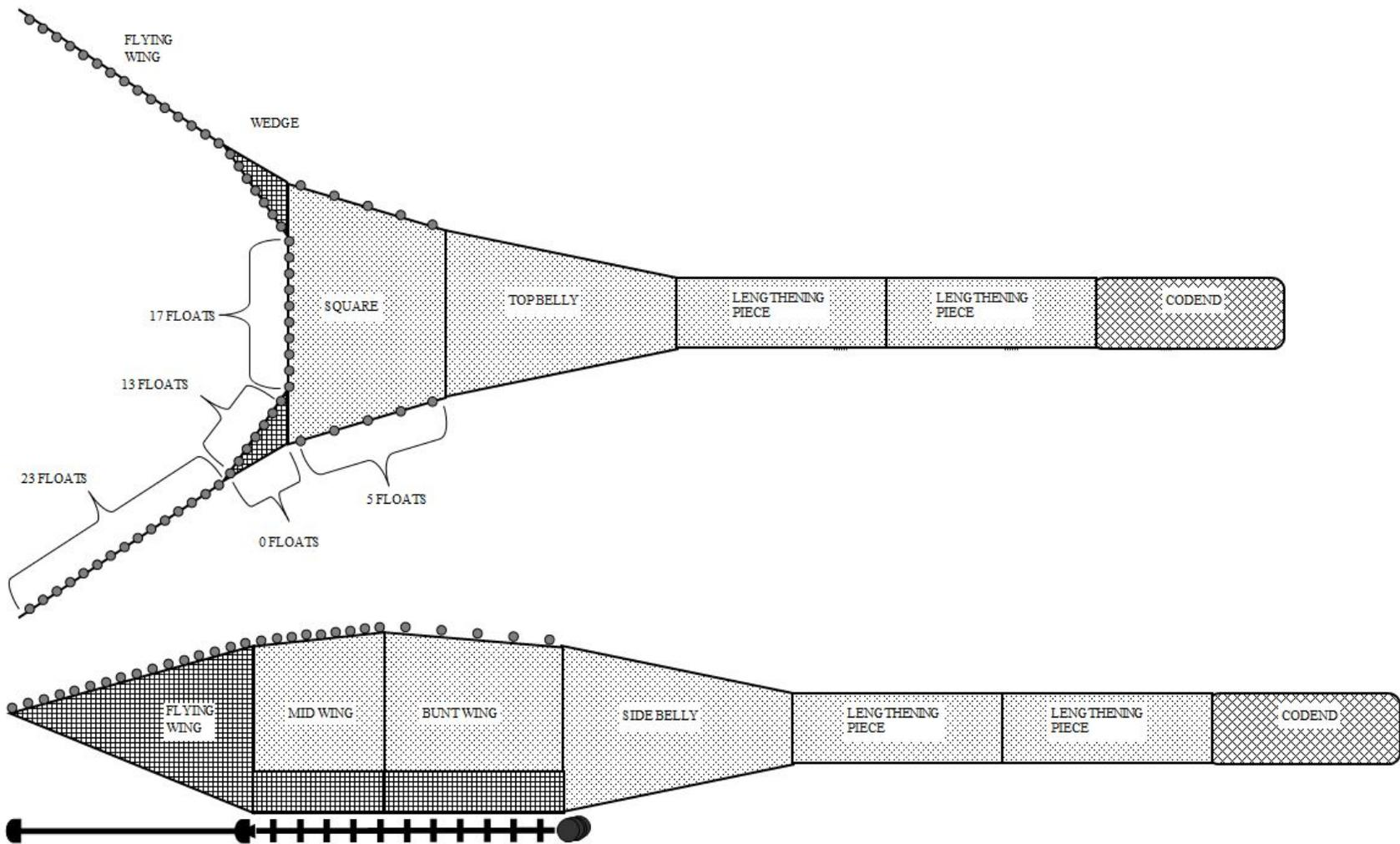
Figure 4. Top and side view of the Atlantic Western Iia box trawl used on the 2016 WCVI synoptic bottom trawl survey.
