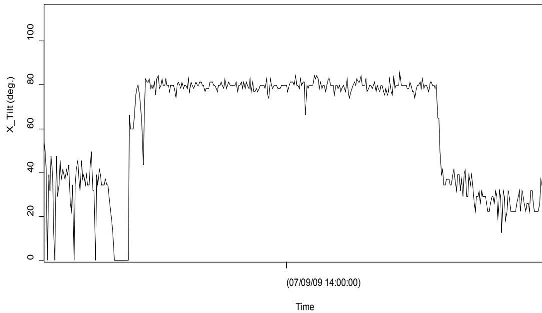
Figure 14. Example of a bottom contact sensor profile collected during a synoptic bottom trawl survey. The raised segment in the middle of the profile at approximately 80° indicates where the net made contact with the sea floor.
