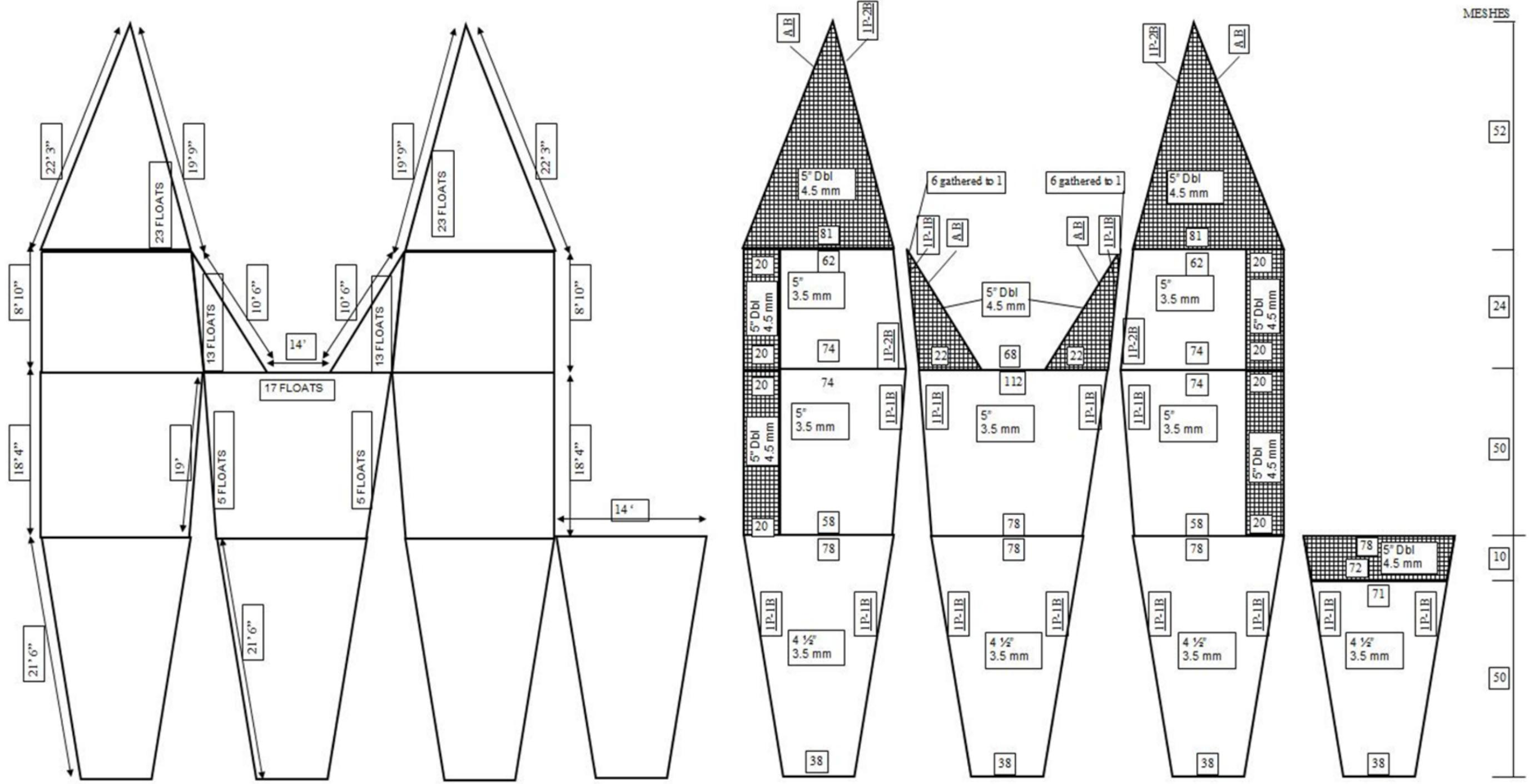
Figure 6. Details of the wing and belly sections of the Atlantic Western Ila box trawl used on the 2016 WCVI synoptic bottom trawl survey. Dimensions and the float arrangement are shown on the left while netting details, mesh counts, and mesh cuts are shown on the right side of the diagram.
