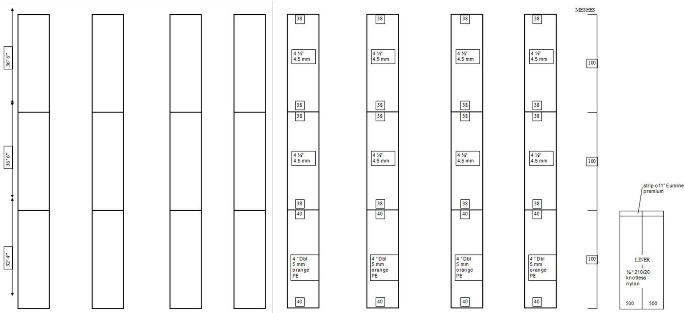
Figure 7. Details of the lengthening (intermediate) pieces and codend sections of the Atlantic Western IIA box trawl used on the 2016 WCVI synoptic bottom trawl survey. Dimensions are shown on the left while netting details, mesh counts, and mesh cuts including the codend liner are shown on the right side of the diagram.
