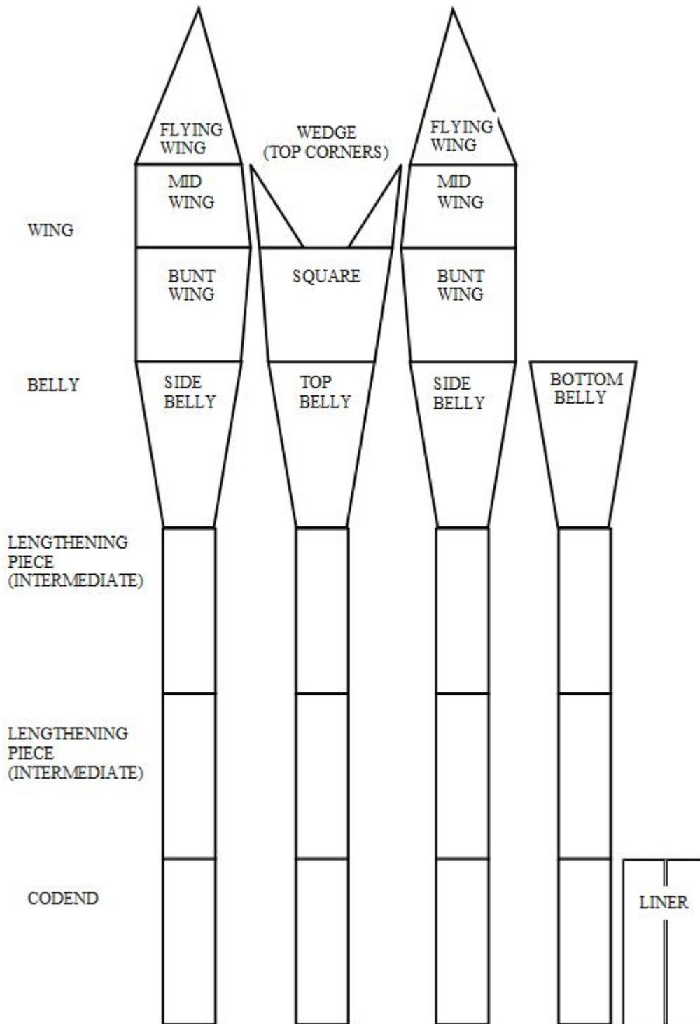
Figure 5. Diagram of the net panels with section names for the Atlantic Western IIa box trawl used on the 2016 WCVI synoptic bottom trawl survey.
