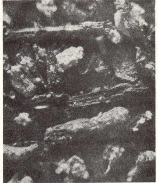
FIG. 19 - ORGANIC MATERIAL IN CORE FROM POND INLET
