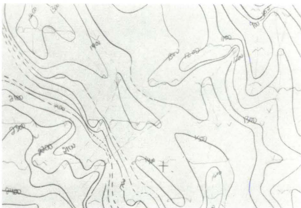
Figure 9: Disagreement between numerically generated contours and features, trends, delineated by the echograms.
