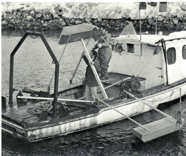
FIG. 9 TRANSDUCER FLOAT SECURED FOR STEAMING
