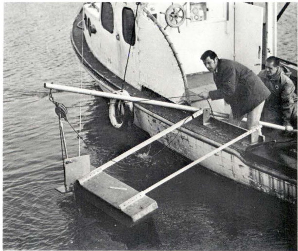
FIG. 14 CALIBRATION OF OUTBOARD SOUNDER
