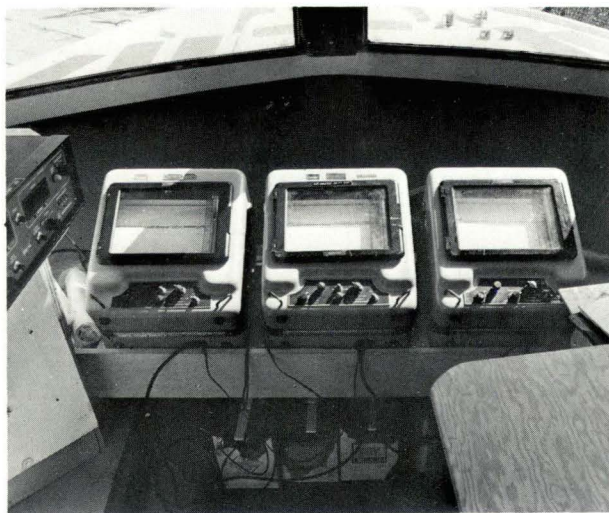
3 SOUNDERS INSTALLED ONBOARD CSL DUNLIN MAY 1977
