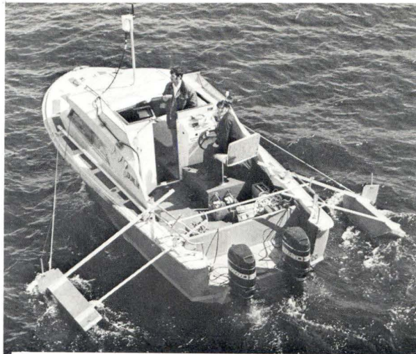
FIG. 7 SWEEP SYSTEM ON CSL DUNLIN
