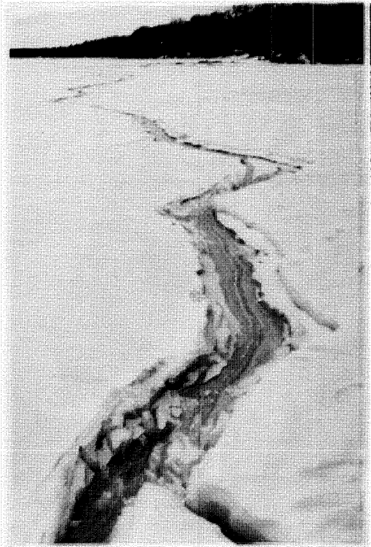
Figure 46. 'Wet' cracks formed by the thermal contraction of an ice cover: (a) the pattern of wet cracks on a small lake in early fall; (b) a refrozen wet crack in late winter.
