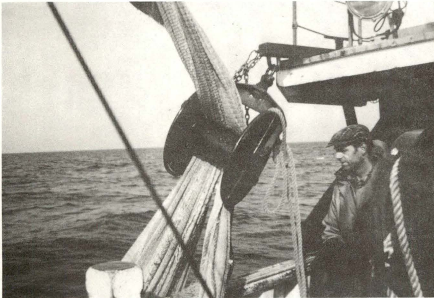
Closeup of dry-up spool, with Mate Wilbert d'Entremont of the "Lady Anna" watching as he hoists a "split" aboard.
