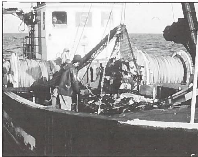
Self-hauling rope reels aboard "The Monique H" off New Brunswick
