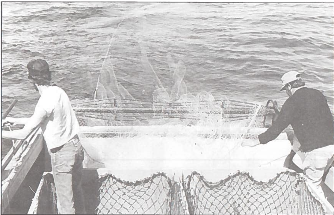
Modified roller (using steel spindle) at stern of a gillnetter
