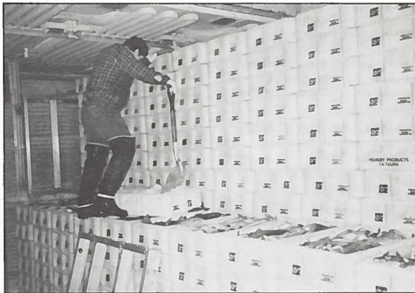
Stromberg 90-litre boxes in use onboard the Fishery Products Stern Trawler Zamberg (53 m). The Zamberg was built in Marystown, Newfoundland, in 1981.
