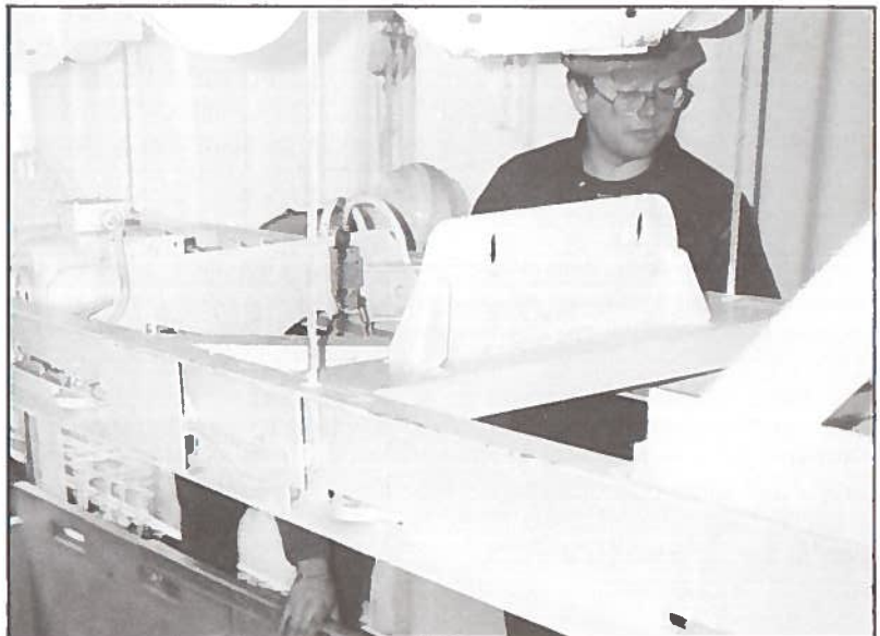
An in-hold view of the travelling bridge and its set of three containers. These can be both manipulated and stored in the fishhold.
