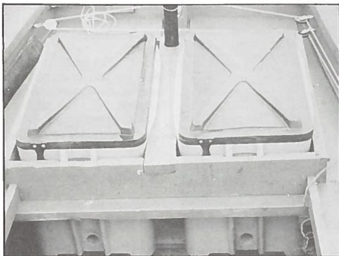
Each of these containers can hold approximately 450 lbs. of round cod, can be moved with ease (note the fork lift adapters on the bottom), and has drainage holes which allow the catch to drain on board.
