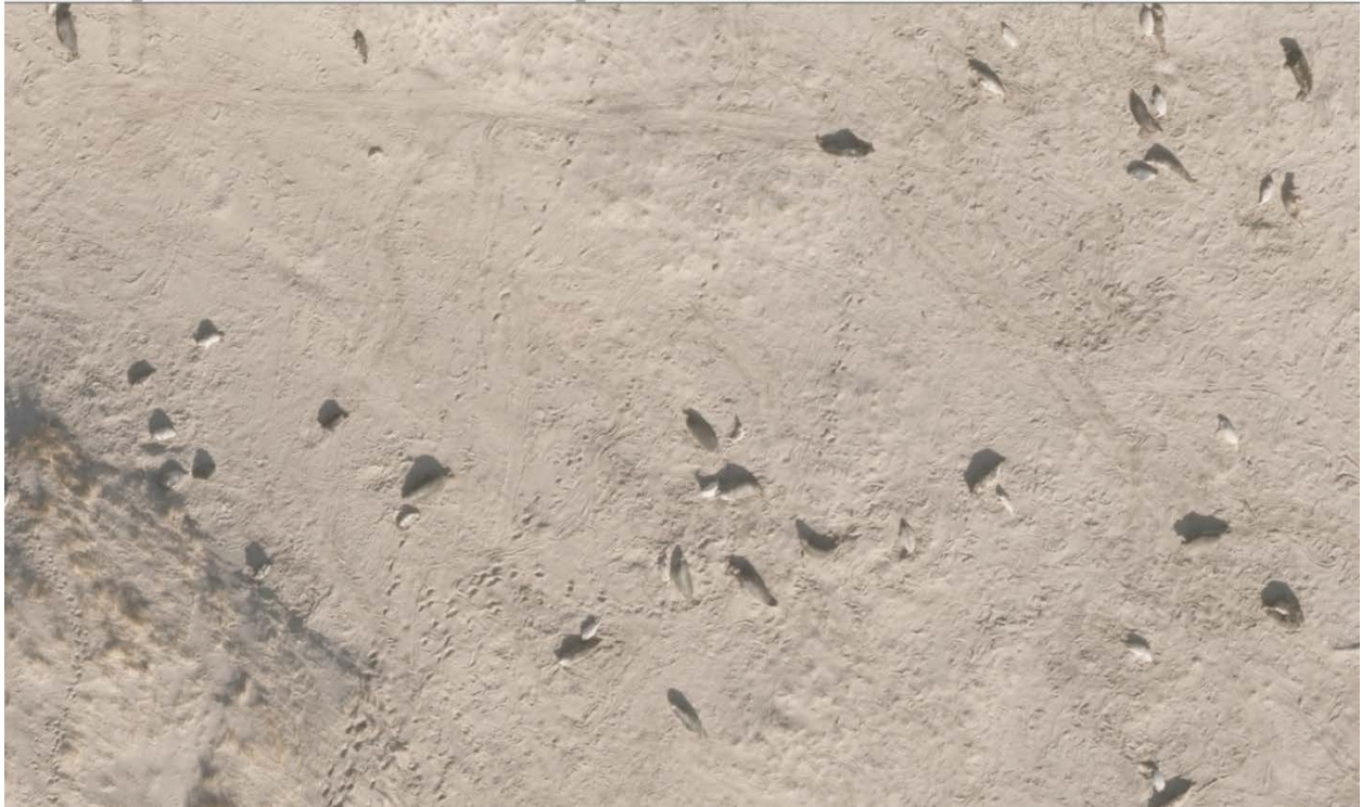
Figure 5. Aerial photographs taken from an altitude of approximately 420 m, using a large format aerial survey camera (Microsoft Vexcel UCX camera) in a motion compensation camera housing.
