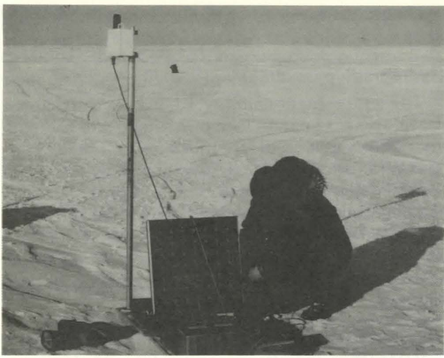
Figure 3. Mini Ranger Solar Powered Positioning System
