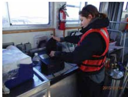
Lindsay Brager (DFO) conducting field tests of a new method for rapidly and accurately measuring sediment sulfide concentrations. Photo: Peter Cranford (DFO)
