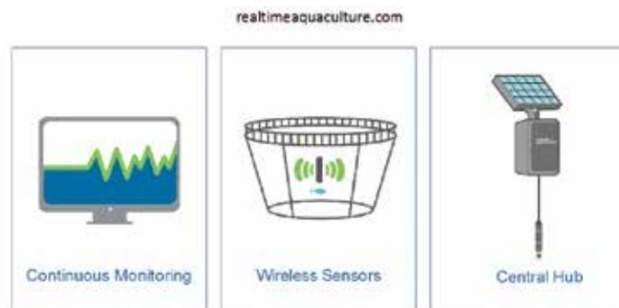
Sensor collaboration with Vemco Amirix ([realtimeaquaculture.com](http://realtimeaquaculture.com)) on cage-specific oxygen and temperature data, with wireless acoustic data logging and smartphone monitoring.
