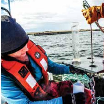
Collecting sediment trap samples for suspended particle analyses. Photo: Kristy Hugill (DFO)
