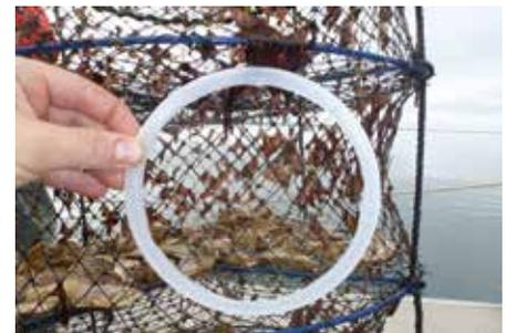
Structure which received an antifouling coating treatment. Photo: Merinov
