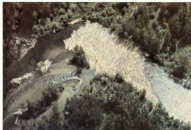
FIGURE 14—Large log jam (partially removed) in Area IX. Note bed load deposits downstream (light color, left side of picture).
