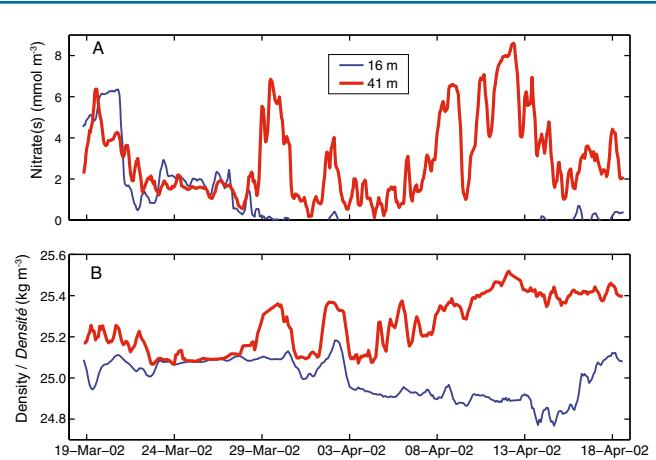
Fig. 3 (A) Nitrate concentrations measured by NAS-2EN instruments at the depths of 16 m (thin line) and 41 m (thick line) at HL2 for the period 18 March 2002 - 18 April 2002; (B) seawater density at depths of nitrate sensors (thin line: 16 m; thick line: 41 m).
