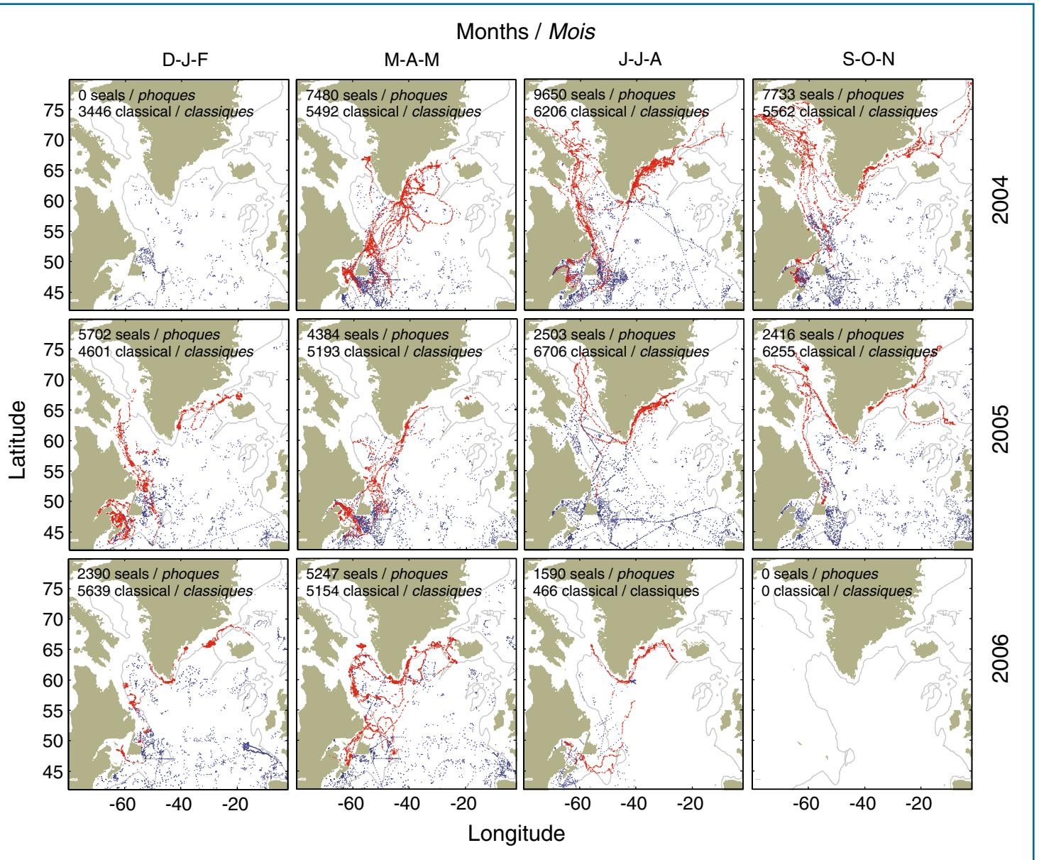
Fig. 2 Location of seal-based temperature profiles/tracks (red) and classically observed profiles (blue) for the North Atlantic (north of 40°N).
