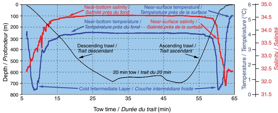
Fig. 3 A typical time series of depth, temperature, and salinity from a 20-minute fishing tow to approximately 700 m depth.
