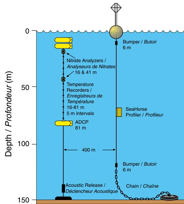
Fig. 1 Schematic diagram of moorings at HL2. The SeaHorse profiles between the lower and upper bumpers every two hours making CTD, fluorometer, and PAR measurements. The second mooring includes two in situ nitrate analyzers, 14 temperature recorders (black circles), and an upward-looking ADCP at mid-depth sampling every 15 minutes.
