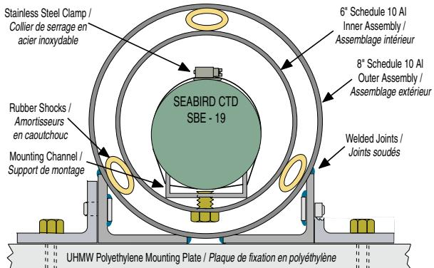
Fig. 1 A cross-section schematic of the shock-absorbing CTD sled showing its major components (Adapted from the original engineering drawings by T. Foulkes, DFO, 1989).
