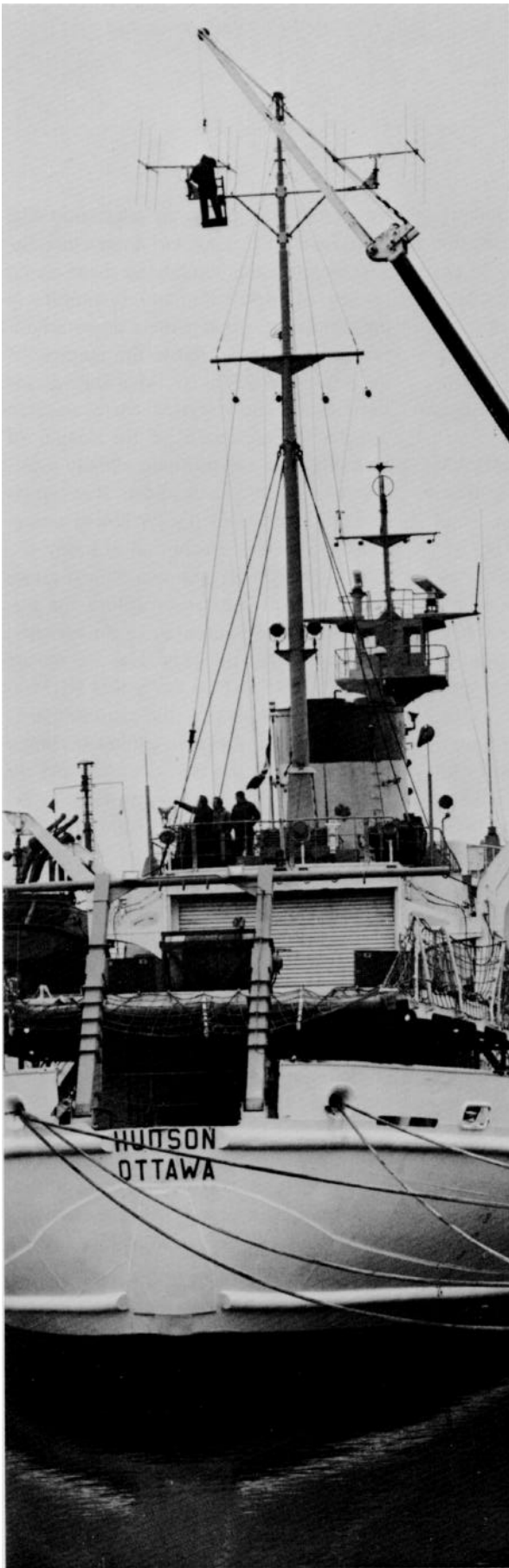
High gain VHF radio antennas being mounted to the aftermast of CSS Hudson . They receive signals from sonobuoys used in geophysical studies.
