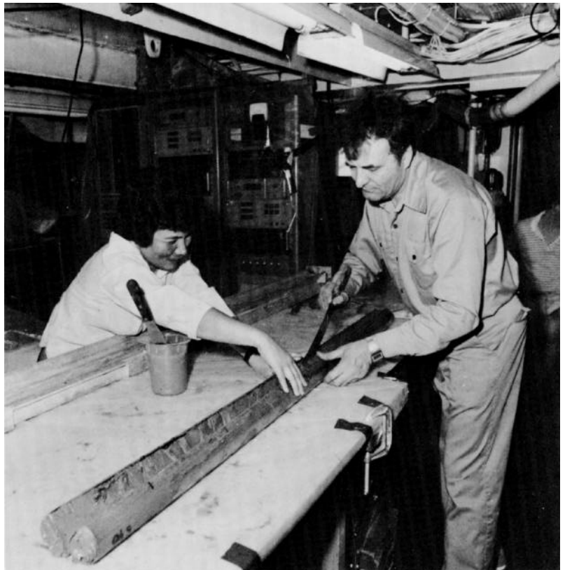
Wang Ying and Gus Vilks split a deep-sea sediment core aboard CSS Hudson . One half the core will be subsampled and analyzed; one half will be archived.
