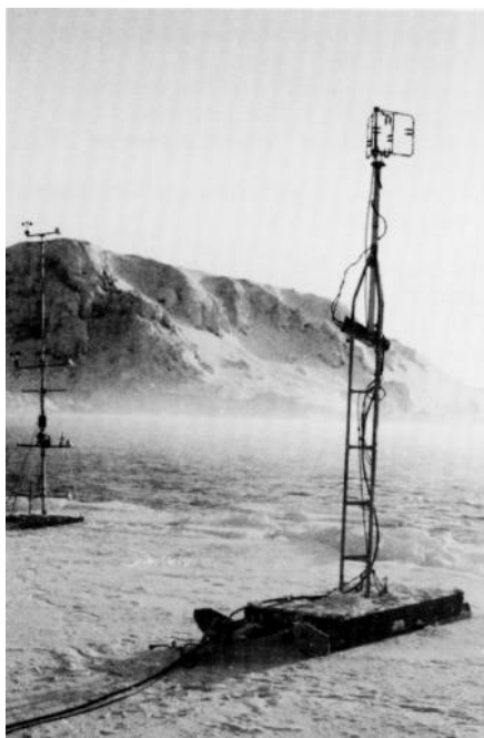
Sonic anemeters set up near the polynya at Dundas Island (near Devon Island) to measure heat flux and wind speed.
