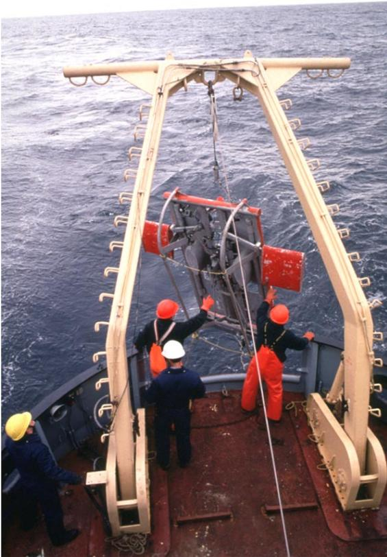
Figure 2. BRUTIV, a towed vehicle used to collect video imagery of seabed habitat.
