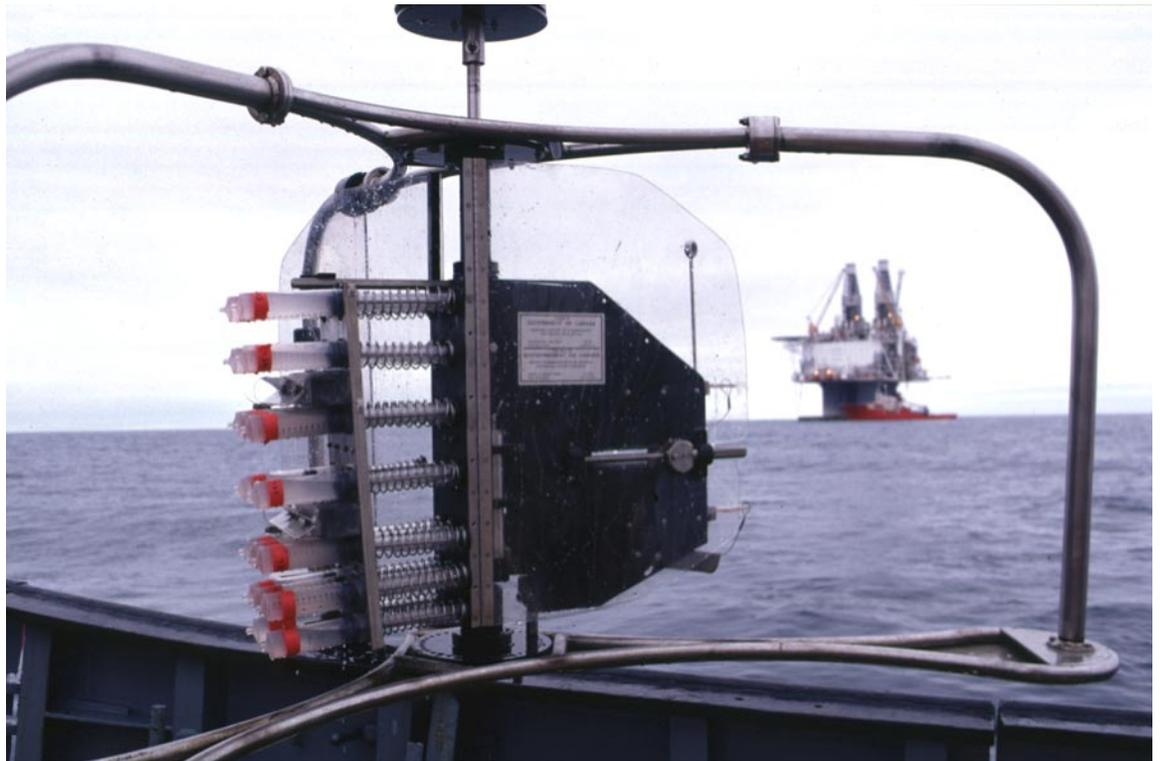
Figure 3: BOSS being recovered after sampling near the Hibernia Platform on the Grand Banks. Suspended sediment samples are collected from the benthic boundary layer by spring loaded syringes at 7 depths between 5 and 50 cm above the sea floor.
