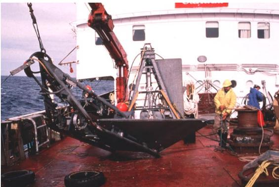
Figure 3. Epibenthic sled which collects large organisms living on the seabed (samples approximately 18 m<sup>2</sup> on a 50 m tow).
