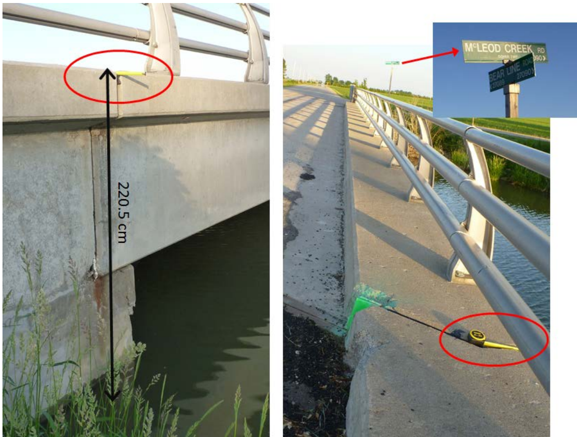
Figure 2. The water surface height relative to the McLeod Bridge was measured on June 3, 2015 at 20:15. The observed distance from the top of the concrete step (beside rubber expansion gap) was 220.5 cm.
