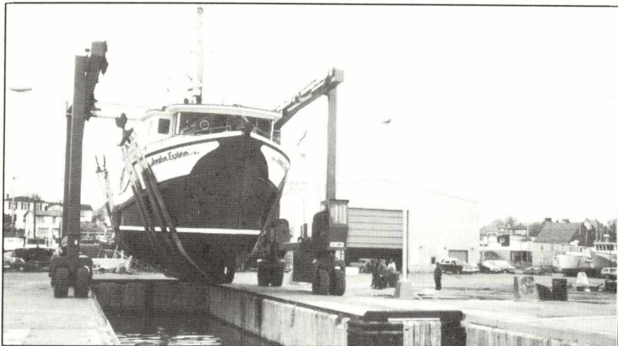
Marine Service Centre straddle cranes make light work of moving longliners into and out of the water.
