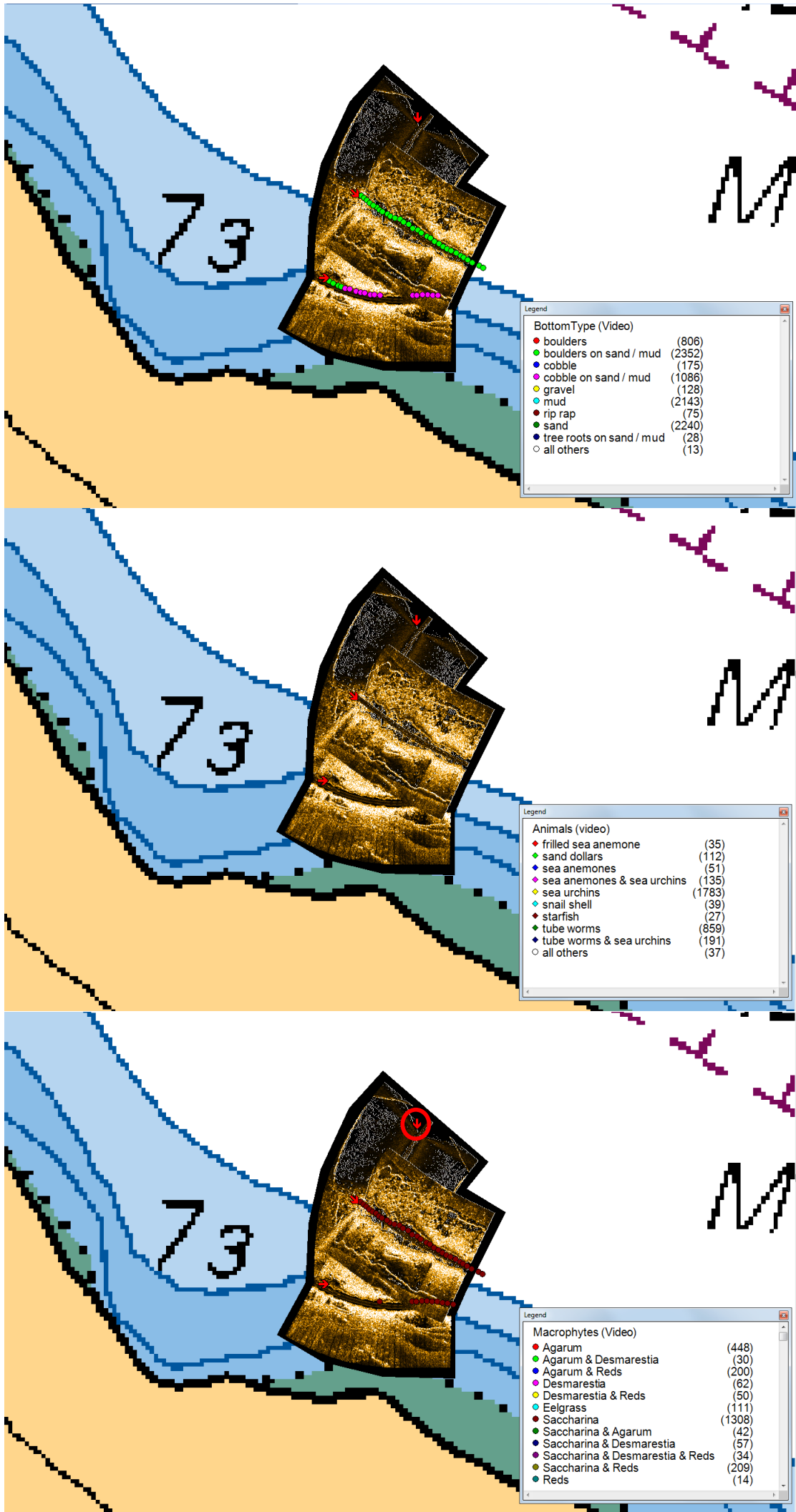
Figure 65: Transect IH25 showing towfish classification results. The red arrow start point for the main transect run (perpendicular to shore) is circled in red and located at 44.632792N 63.601908W.
