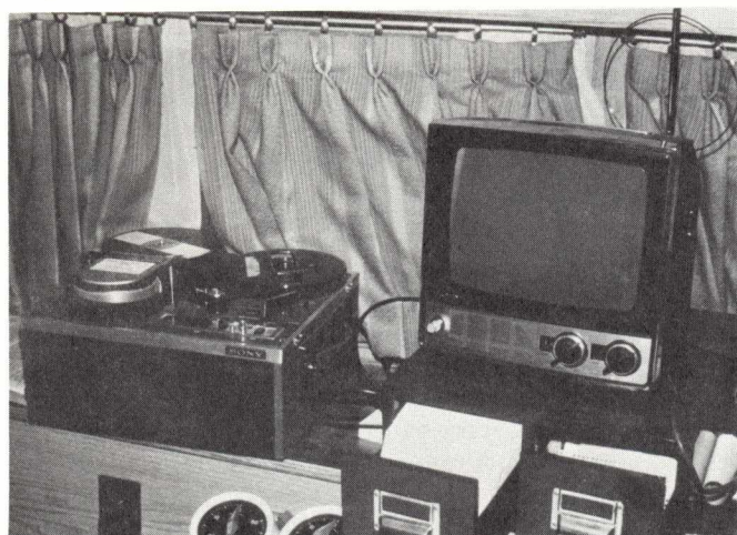
Video tape recording and timing instrumentation for automatically counting downstream-migrant alewives through the bypass at Tusket Falls hydroelectric development.
