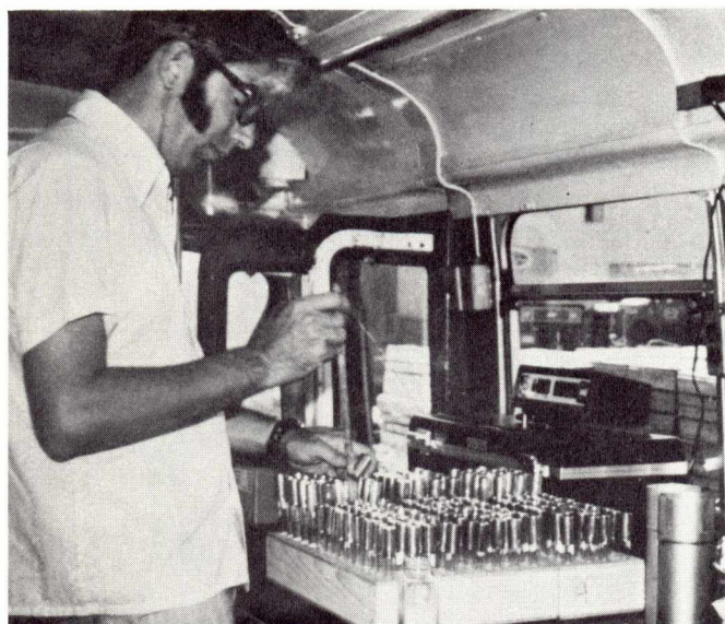
Bacteriological sampling by the multiple-tube dilution test, to evaluate coliform bacteria level in clams.
