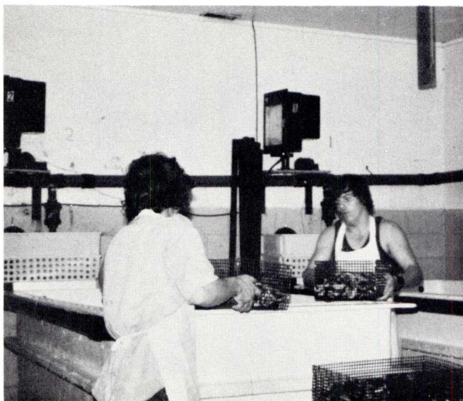
Loading baskets of soft-shell clams into a depuration tank.
