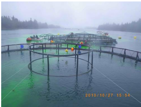
Figure 3: A series of photographs showing the temporal evolution of dye, and hence therapeutant, leaving a tarped fish cage. The photographs were taken just prior to the beginning of flushing (top left), 5 minutes (top right), 10 minutes (middle left), 15 minutes (middle right), 20 minutes (bottom left) and 24.5 minutes (bottom right) after flushing began.
