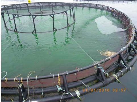
Figure 4: A second series of photographs showing the temporal evolution of dye, and hence therapeutant, flushing from a different tarped fish cage. The photographs were taken just prior to the beginning of flushing (top left), and 20 minutes (top right), 50 minutes (middle left), 80 minutes or 1.3 hours (middle right), 110 minutes or 1.8 hours (bottom left) and 170 minutes or 2.8 hours (bottom right) after flushing began.
