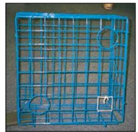
On traps with a rigid frame and a freely opening hinged lid, the trap lid must be secured by a loop of the same type of twine so that the lid will open freely when the rot cord breaks. There must not be any other fastenings that can interfere with the opening of the lid.
