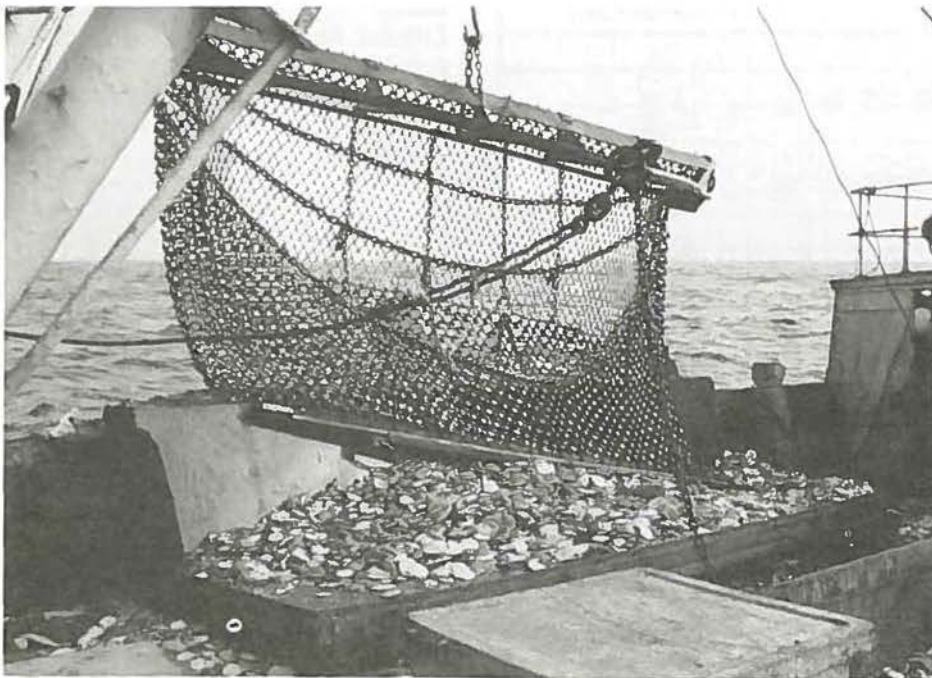
Fig. 6 - Bringing aboard an offshore scallop drag. Empty drag weighs 454 kg, with a full catch as much as 3 600 kg.
