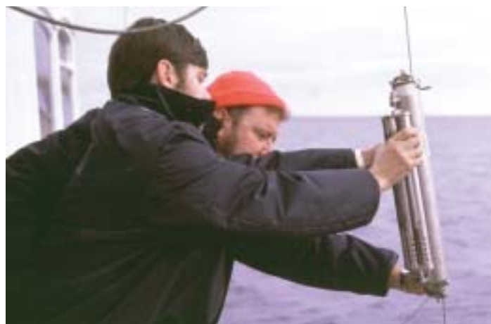
Observing temperature and salinity using a Knudsen bottle and reversing thermometers.
