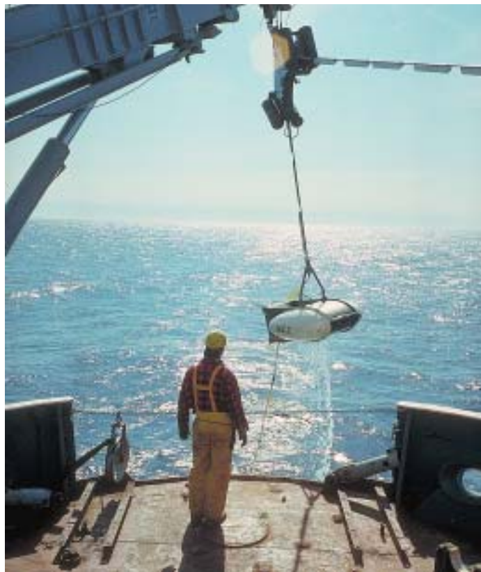
Huntec Deep-Towed Seismic Reflection System (DTSTM) was developed in an industry-BIO partnership in the 1970s, and used throughout the world for deep seismic profiling.
