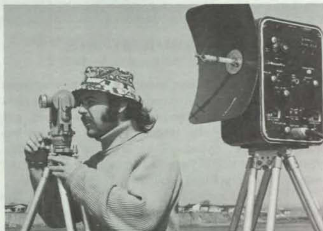
Figure 4. MRB 2 Hydrodist shore station used in range-bearing mode on Lake Huron.
