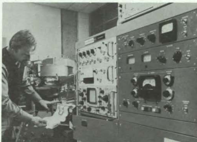
Figure 21. Incorporation of improved system modules to CCIW Hitachi mass spectrometer installation.
