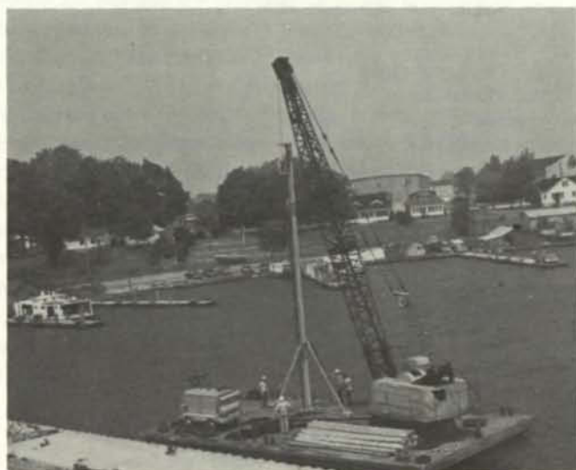
Figure 3. Assembly of the Vibracore sampler, Kingsville Harbour.
