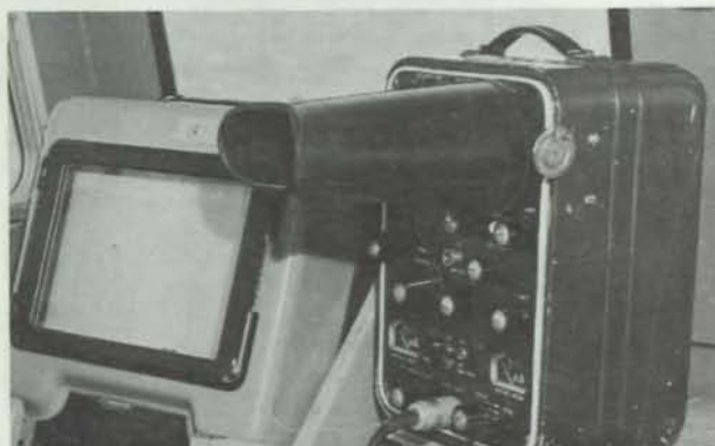
Figure 3. MRB 2 Hydrodist and Raytheon echo sounder used in the St. Lawrence River Survey.
