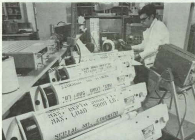
Figure 27. Acoustically triggered underwater release units.
