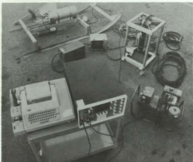
Figure 8. Prototype neutron-activated sediment-tracking system.
