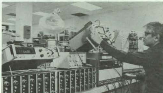
Figure 22. Electronic instrumentation for pre-processing IFYGL Micromet turbulence field data.
