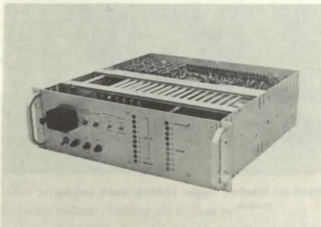
Figure 39. Auto-sequencer for CO 2 monitor system.
