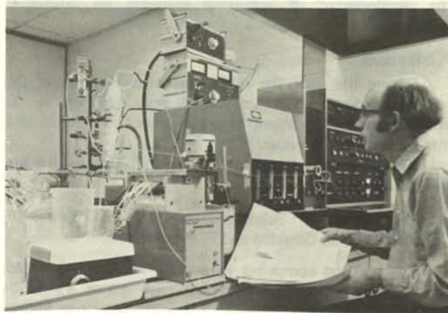
Dr. Peter Goulden observes the flow rates in the simultaneous analysis of selenium and arsenic by atomic absorption spectroscopy.
