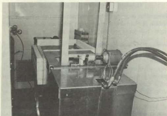
Figure 47. Reverse osmosis membrane manufacturing apparatus.
