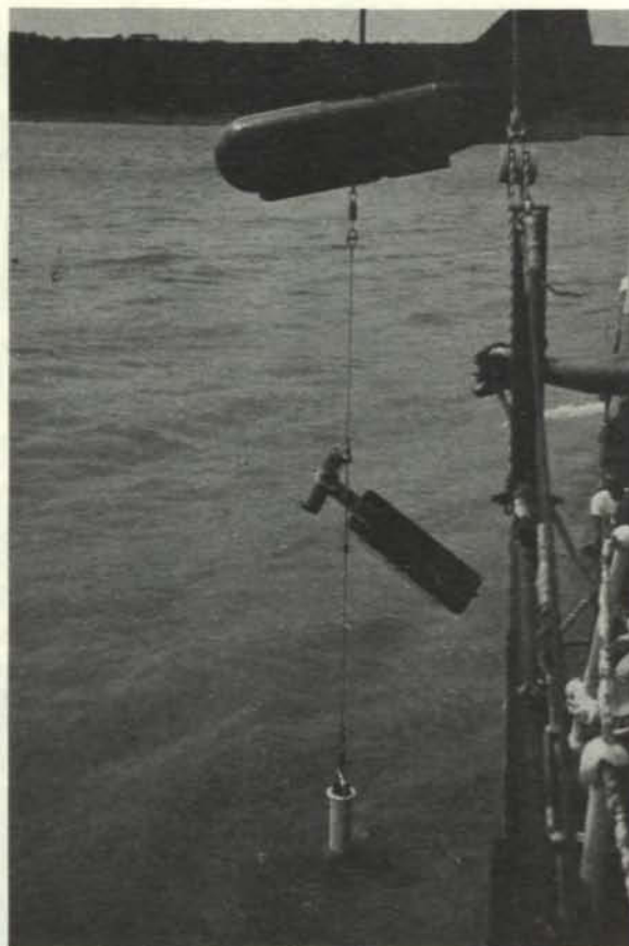
Current meter mooring system showing subsurface float, current meter and acoustic release.
