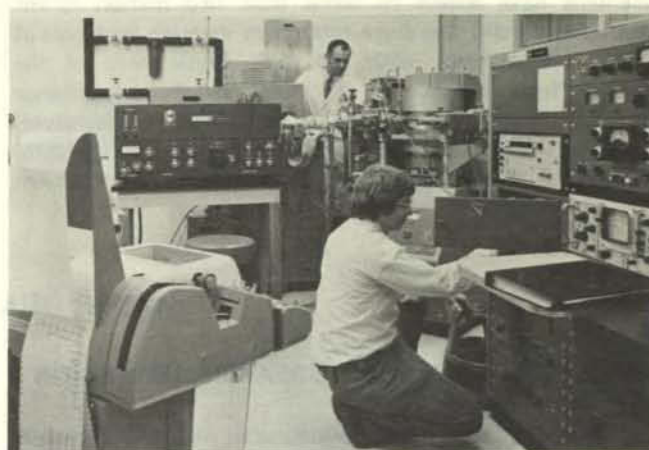
Mike Comba (foreground) and Dr. Frank Onuska check the settings of their Mass Spec/Gas Chromatograph for the identification of pesticide residues.
