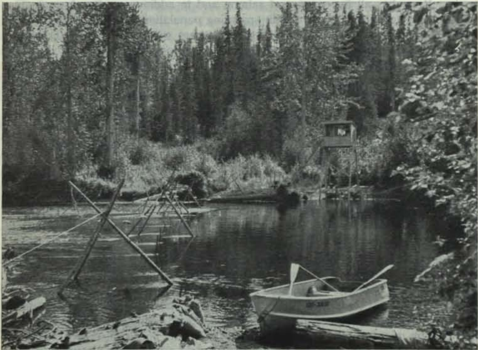
Salmon counting tower. The tripods hold electric light line used for night counts.
