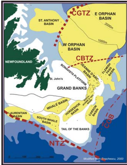
Figure 3. Distribution of Mesozoic sedimentary basins around the Grand Banks. (CGTZ = Charlie Gibbs Transfer fault Zone, CBTZ = Cumberland Belt Transfer fault Zone, NTZ = Newfoundland Transfer fault Zone, COB = Continent-Ocean Boundary). Source: (Enachescu & Fagan, 2005).
