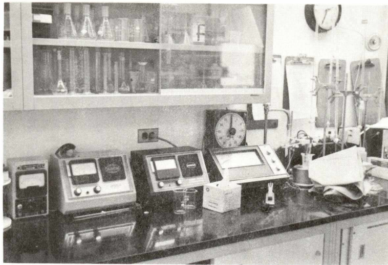
Fig. 21. Some laboratory instrumentation, pH, conductivity, and turbidity meters.
