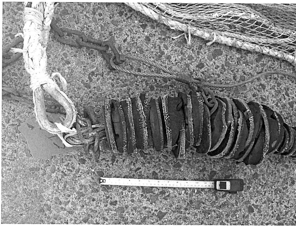
Appendix Figure 4. Corners of the footropes of the two nets used in the net calibration experiment aboard the CCGS *Neocaligus*, August 22-23, 2004. A) Lingcod survey footrope; B) Shellfish survey footrope.
