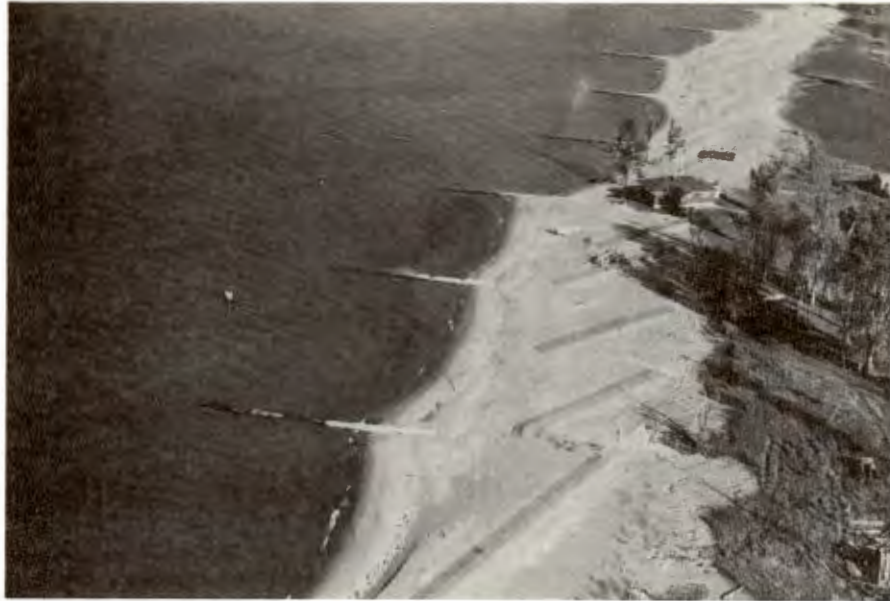
Plate 3. AERIAL PHOTOGRAPH SHOWS DRIFT ACCUMULATION ON WEST SIDE OF GROYNES, INDICATING A REVERSAL IN LITTORAL CURRENT. (PHOTOGRAPHED OCTOBER 20, 1978)
