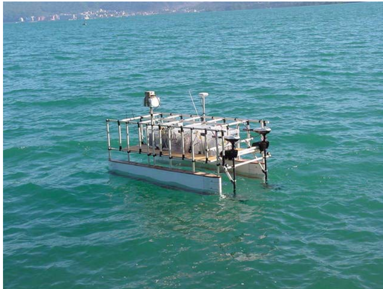
Fig. A SWATH type robot boat with styrofoam twin hull constructed by pipes, operating two electric thrusters. This boat is easy to disassemble, construct, and carry to anywhere in the world.
