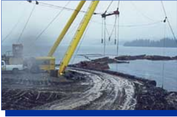
Photo 16. Log dumping using a vertical hoist method
