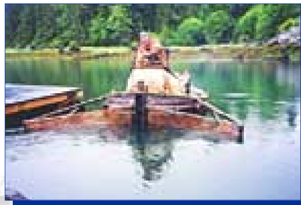
Photo 30. The "sea rake", developed by Triumph Timber Ltd. to collect debris for disposal
