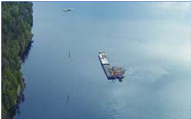
Photo 17. Helicopter log drop, directly to a barge
