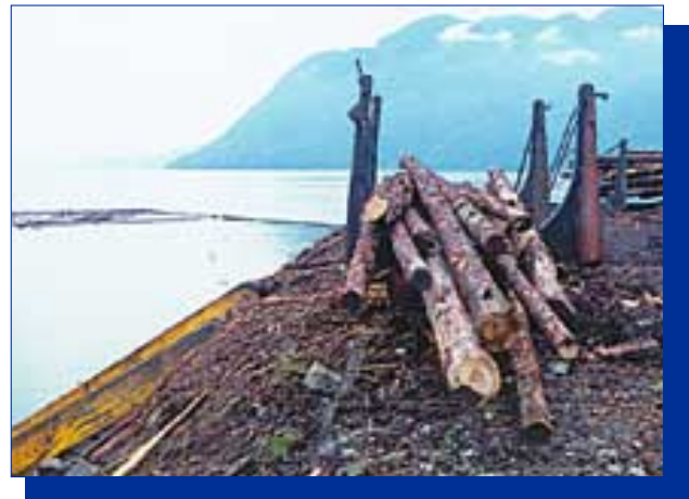
Photo 15. Log dump using steel skids on steep shoreline
