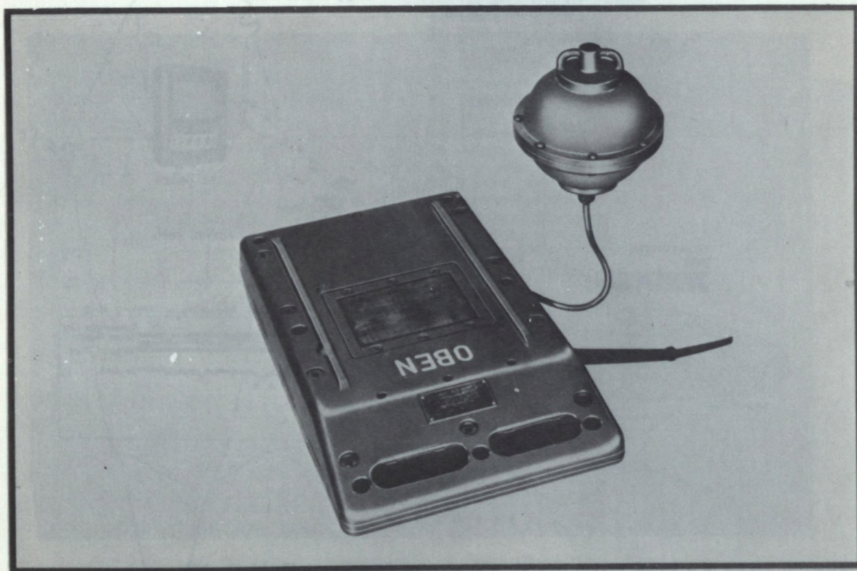
Figure 14 Multi-netsonde transducer board with temperature sensor. (Fried. Krupp GmbH, Atlas Electronic, Bremen)
