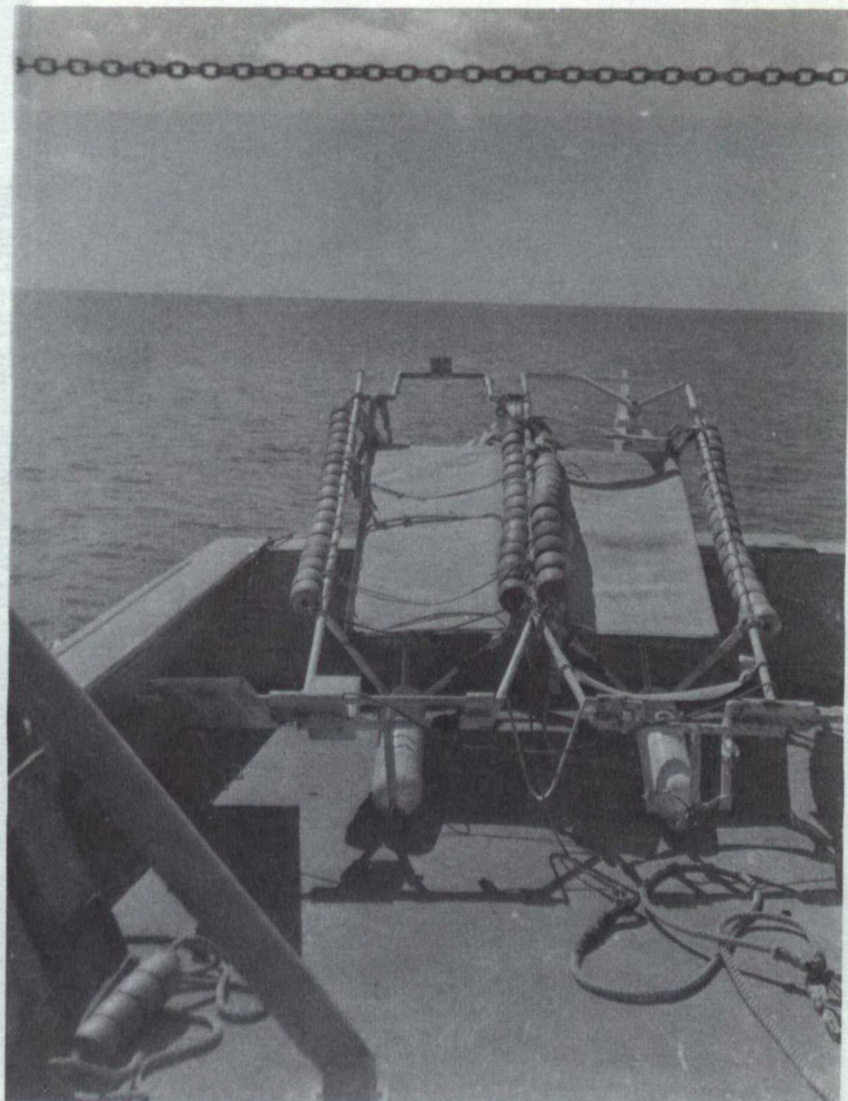
Figure 10 Two men diver's sled for trawl observations. (U.S. Fish and Wildlife Service, Pascagoula Fishery Station)
