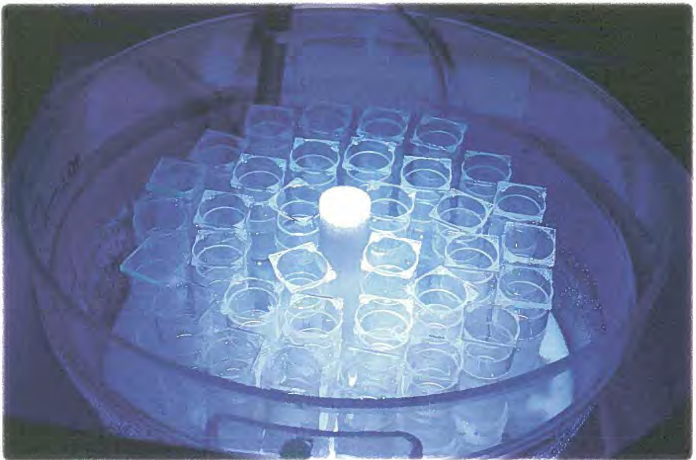
Cod eggs in quartz tubes subjected to radiation from a solar simulator.
