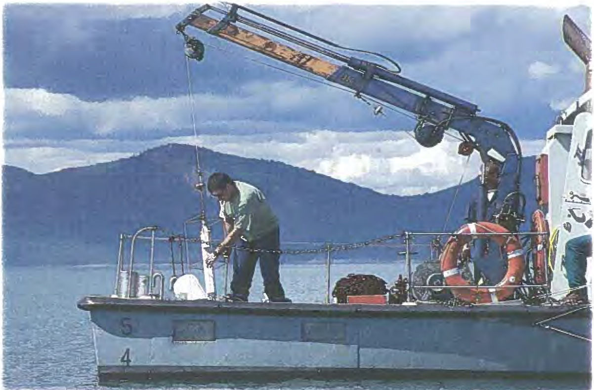
Scientist preparing to deploy an instrument for measuring water temperature, salinity and density between the surface and the bottom.
