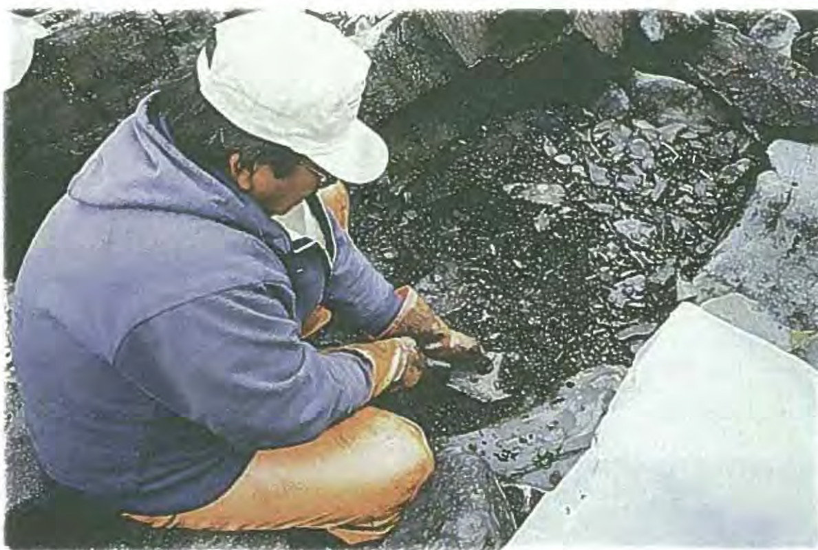
A sample of sediment contaminated by an oil spill is taken for analysis.
