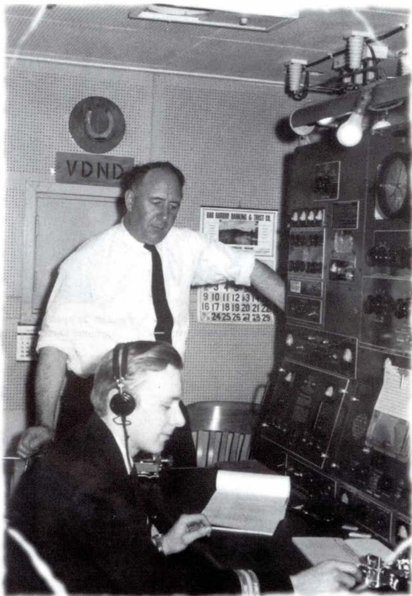
Blue Nose II radio room with radio officers Henry Whitehead (standing) and David Wail. The RCA 5U station was manufactured in the 1950s and installed on the RCMP Wood , the Bounty and the D'Iberville . The RCA unit had a 150-watt output, c. 1965. (David Wail)
