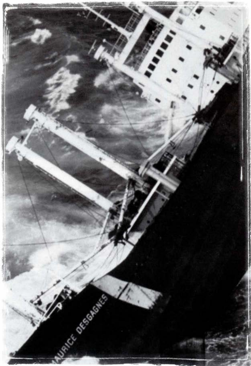
The M/V Maurice Desgagnés just before it sank. On the morning of March 12, 1980, a huge sea struck the M/V Maurice Desgagnés and caused some of her cargo to break loose in the hold. The loose cargo damaged some bulkheads and caused a crack in the deck. Water began to seep in, 1980. (C.F.B. Shearwater)
