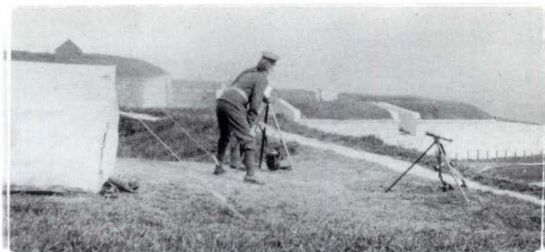
Army personnel using heliograph signalling equipment at the Citadel in Halifax, Nova Scotia. The heliograph was one of the many communications systems used before the advent of wireless telegraphy, c. 1914. (National Archives of Canada, PA112391)
