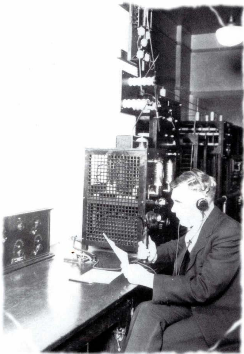
Radio operator Jim Harker operating what was then the new radiotelephone installation of Vancouver radio, VAB, in 1925. The receiver was the famous Northern Electric Peanut tube set. (Courtesy of the S.P.A.R.C. Museum)
