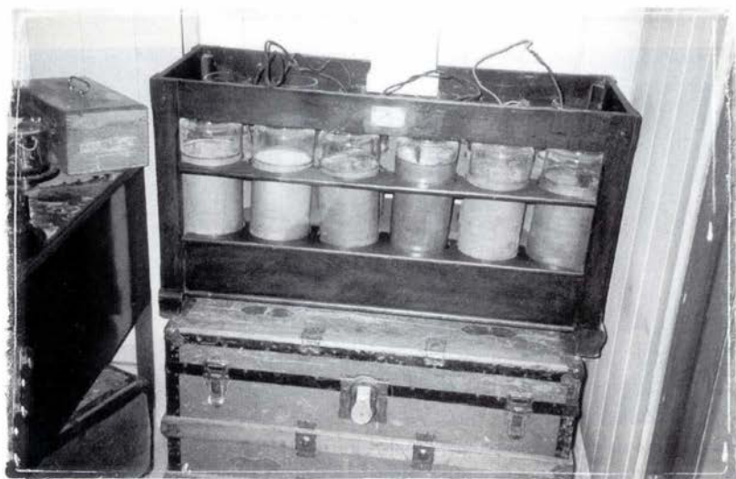
Leyden jars, type of capacitor used with the spark transmitter, 1996. (Courtesy of the S.P.A.R.C. Museum)
