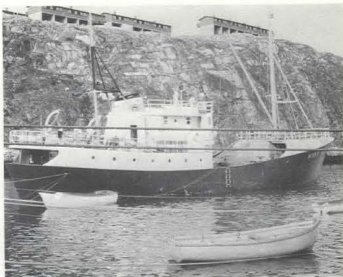
Faeroese and Norwegian (right) salmon drift-netting vessels in West Greenland ports. Three to eight miles of drifting net are set at night from each vessel from August through November, fishing the waters of the West Greenland – Davis Strait area. On such vessels the fish are cleaned and quick-frozen as soon as they are taken from the net. The high-quality product brings as much as $2.50 a pound in European markets.
