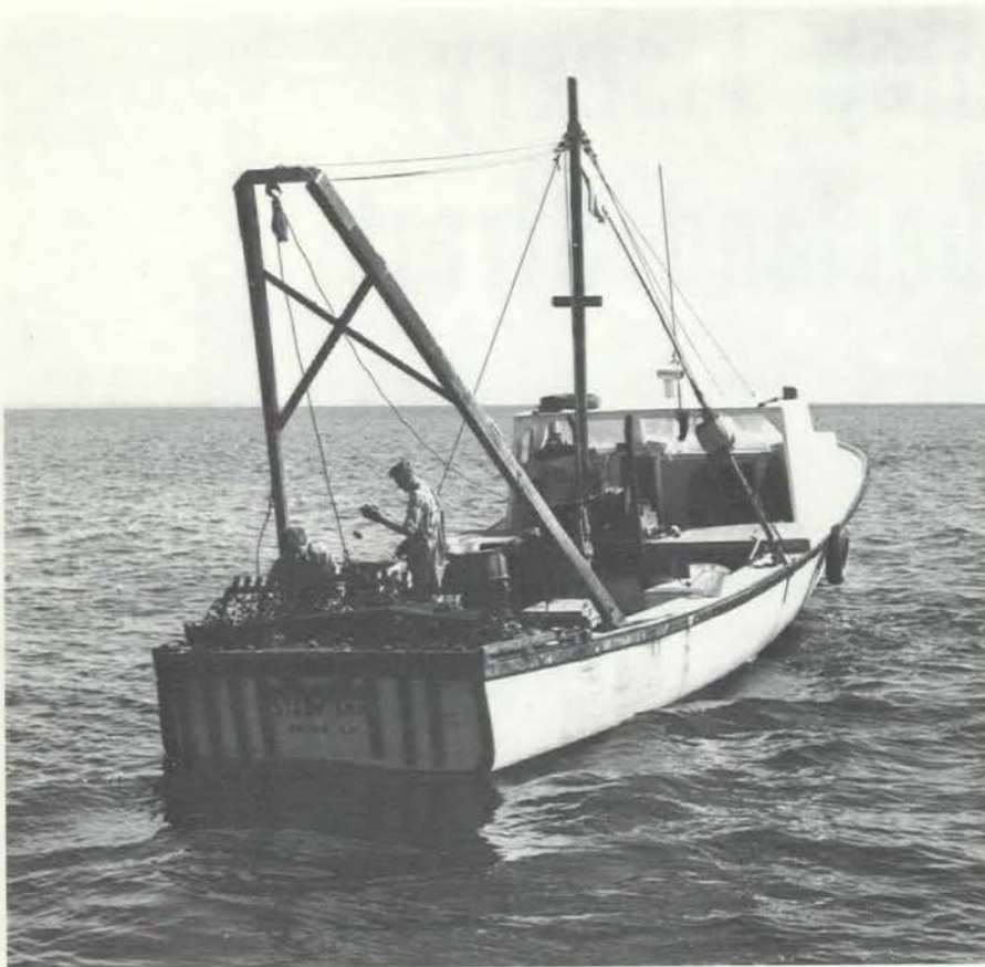
The "Stacy Ann", skippered by Robert Hughton, of Pictou, N.S., is typical of the scallop boats operating in the Northumberland Strait. This vessel is equipped with an "A" frame-type drag.
