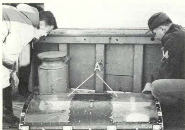
Figure 2: Underwater case containing camera and flash units designed to reduce distortion to the net. Pictures are taken through clear plastic windows (A) in the case.
