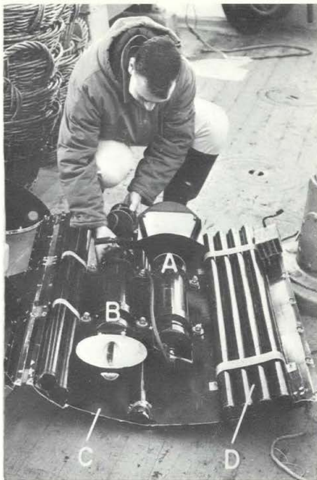
Figure 1: Preparation of multi-exposure camera (A) and electronic flash (B) before the case (C) is attached to headline of an otter trawl. Buoyancy tubes (D) reduce weight of unit in water.
