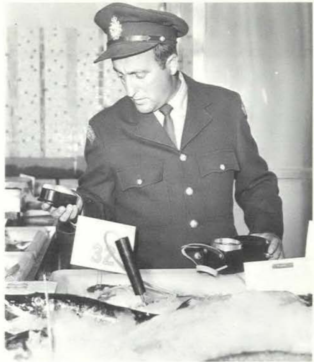
Inspection Officer Paul G. Houle checks the internal temperature of fresh fish in a Montreal fish market with a resistance thermometer.
