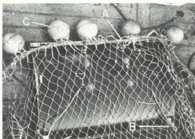
Figure 3: Underwater case shackled to headline (A) and square (B) of an otter trawl. The floats (C) attached to the headline are a normal part of the trawl.
