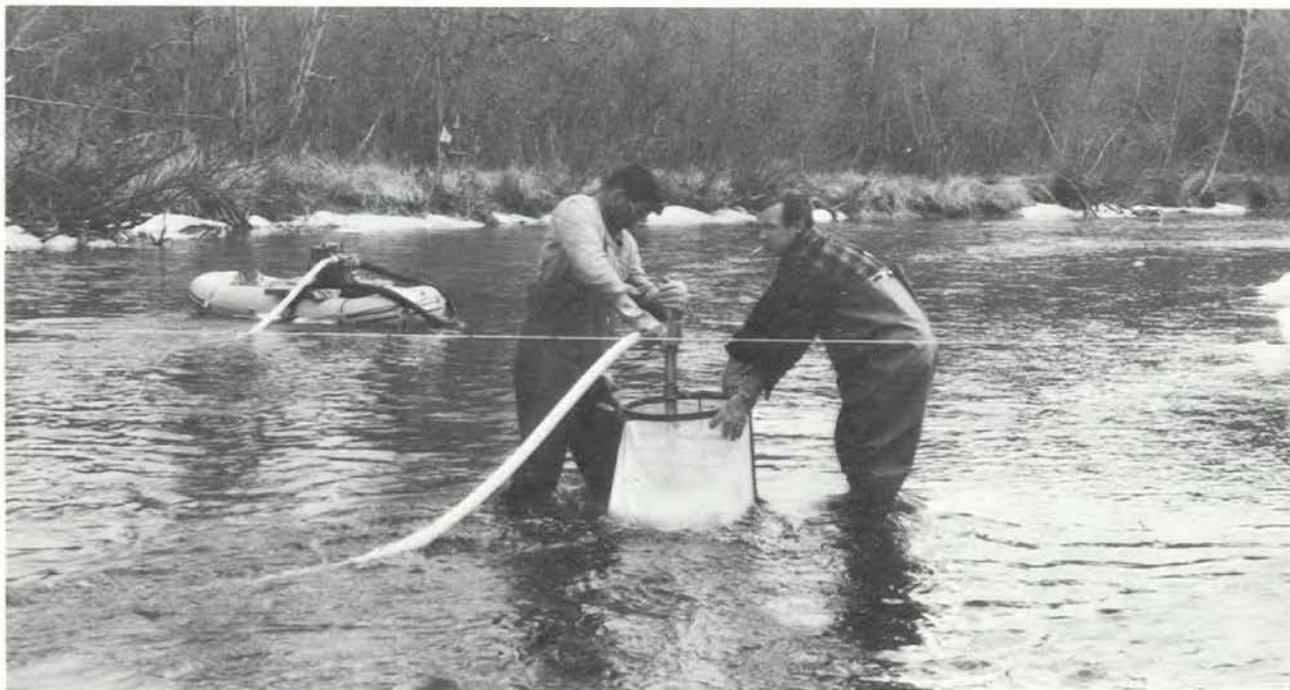
Estimating fry survival at Pinkut Creek by means of hydraulic sampler technique, 1965.
