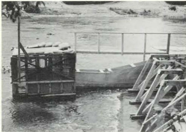
An improved smolt trap on the Miramichi River; screens in the bottom of the flume from the fence to the trap divert most of the water and prevent damage to the smolts from excessive turbulence.
