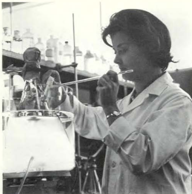
This apparatus at the Vancouver Technological Laboratory is used to grow marine phytoplankters in mass culture. Such culturing requires continuous illumination and strict temperature control.
