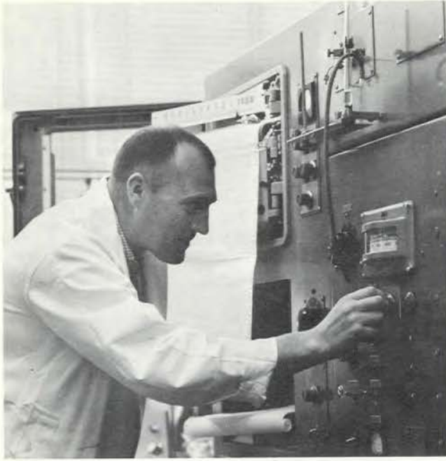
Adjusting the column temperature of an argon detector gas-liquid chromatograph during the analysis of the flavor components of the oyster.
