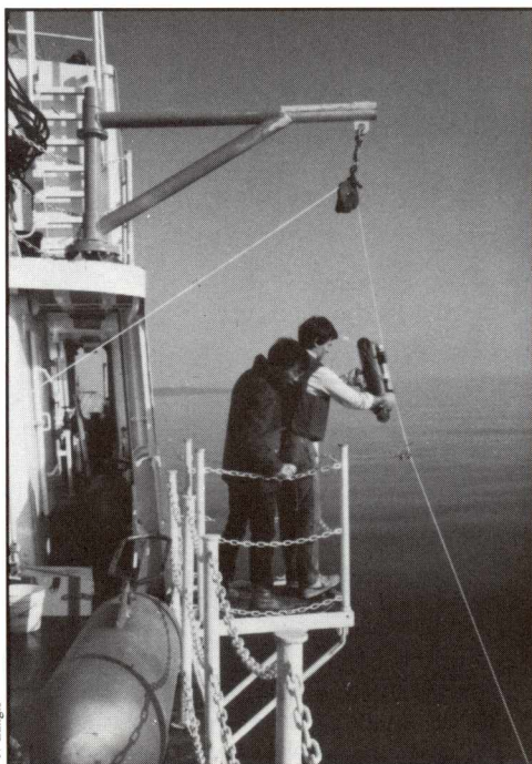
Sampling of water with "Niskin" bottle.
