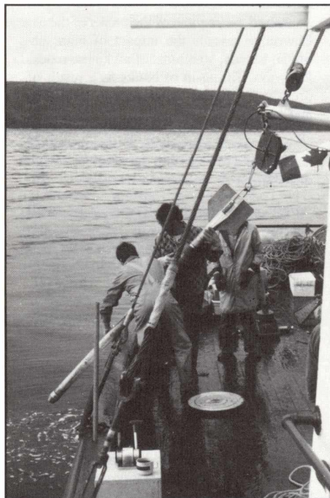
Sampling of marine sediments with a corer permits to accumulate significant data on contamination of fish habitat, and to identify problematic sectors.
