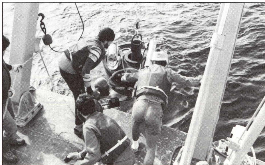
Mooring of measurement line. A tidegauge is put up at left.
