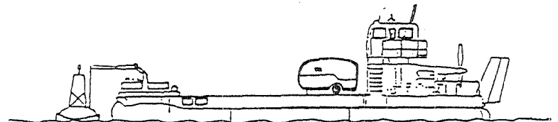
Vehicle in Displacement Buoy Package Installed - Boom Cable Secured to Buoy Crew and Tool Module Installed
