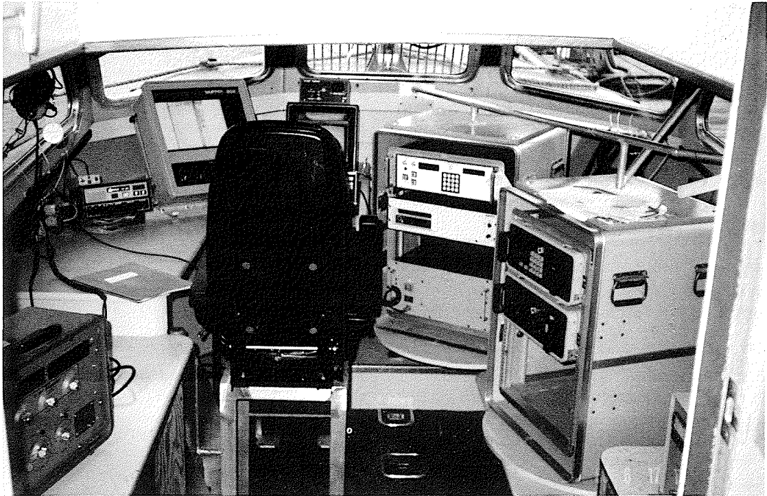
A typical configuration of electronics for inshore hydrographic survey. From port to starboard: distance measuring unit (DMU), VHF radio, Skipper echo sounder, monitor and HAL (hydrographic acquisition and logging) system keyboard, Qantex data storage and tape drive unit (top), MSI depth digitizer, HAL, and ARGO positioning system including the receiver, range positioning and control display units.
