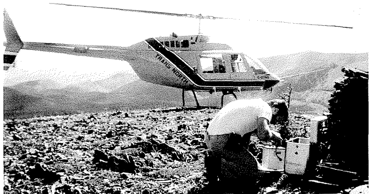
Measuring gravity at a surveyor's cairn in the Ogilvie Mountains, Yukon.
