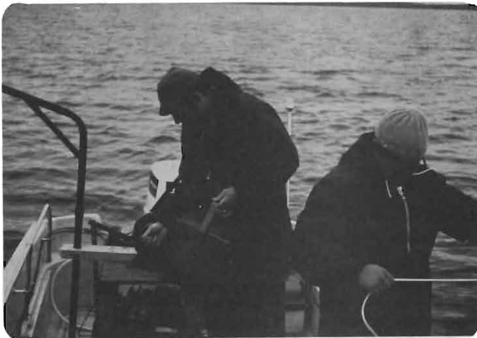
Fig. 10. Benthic sampling using Ekman dredge.
