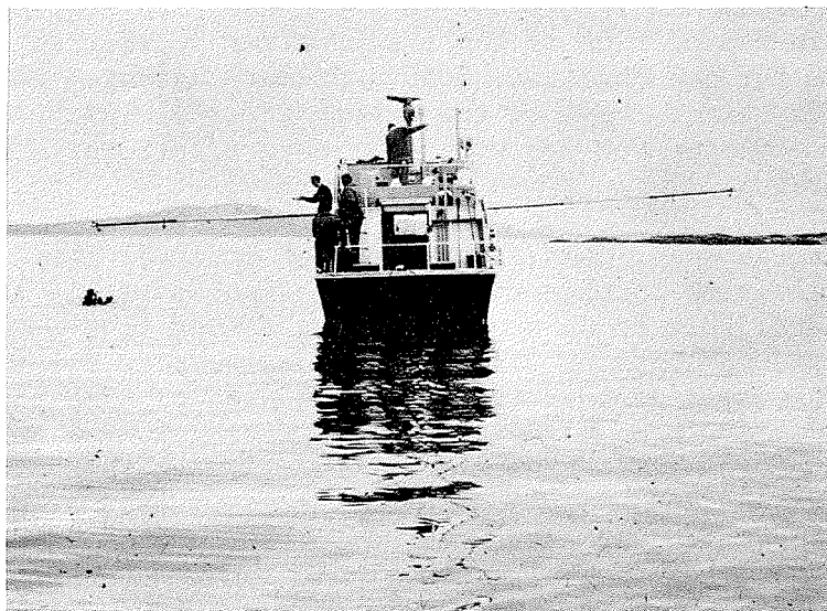
M.V. Revisor at anchor near Discovery Island. Ships' staff have just assembled the sweep apparatus and one of our divers is checking the depth of the wire drag.
