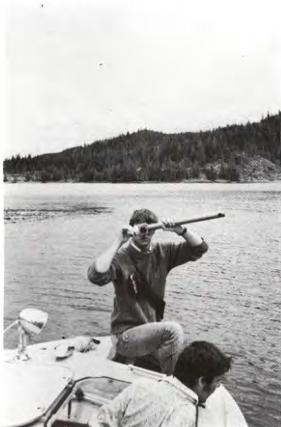
Plate 4. Kelp bed area determination using an optical range-finder.
