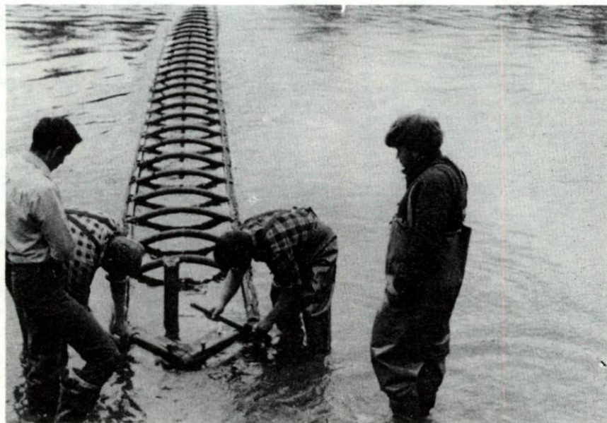
Part of the Bendix acoustical fish counter apparatus on the Lakelse River.
