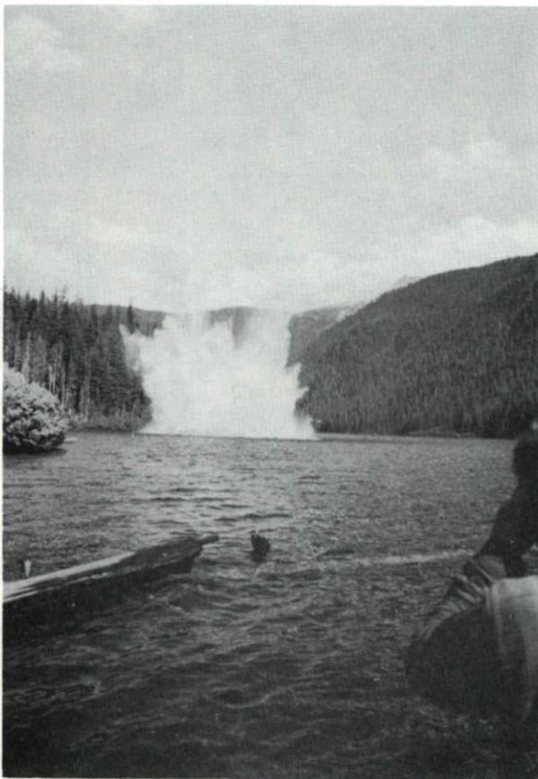
Detonation of a 300 lb. charge at a depth of 40 ft., Greenbush Lake.
