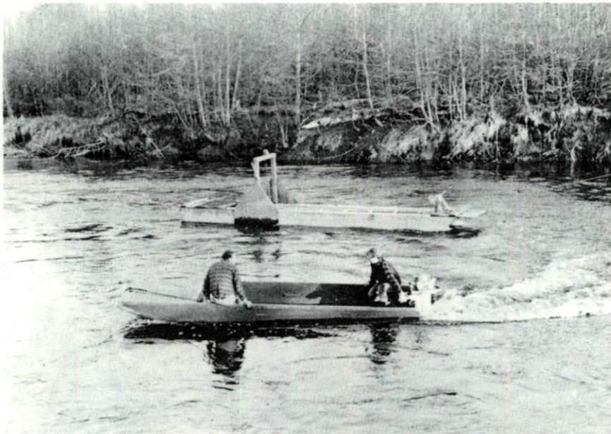
One-foot "wide" inclined plane trap for sampling emigrating juvenile salmonids in fishing position on the Yakoun River.
