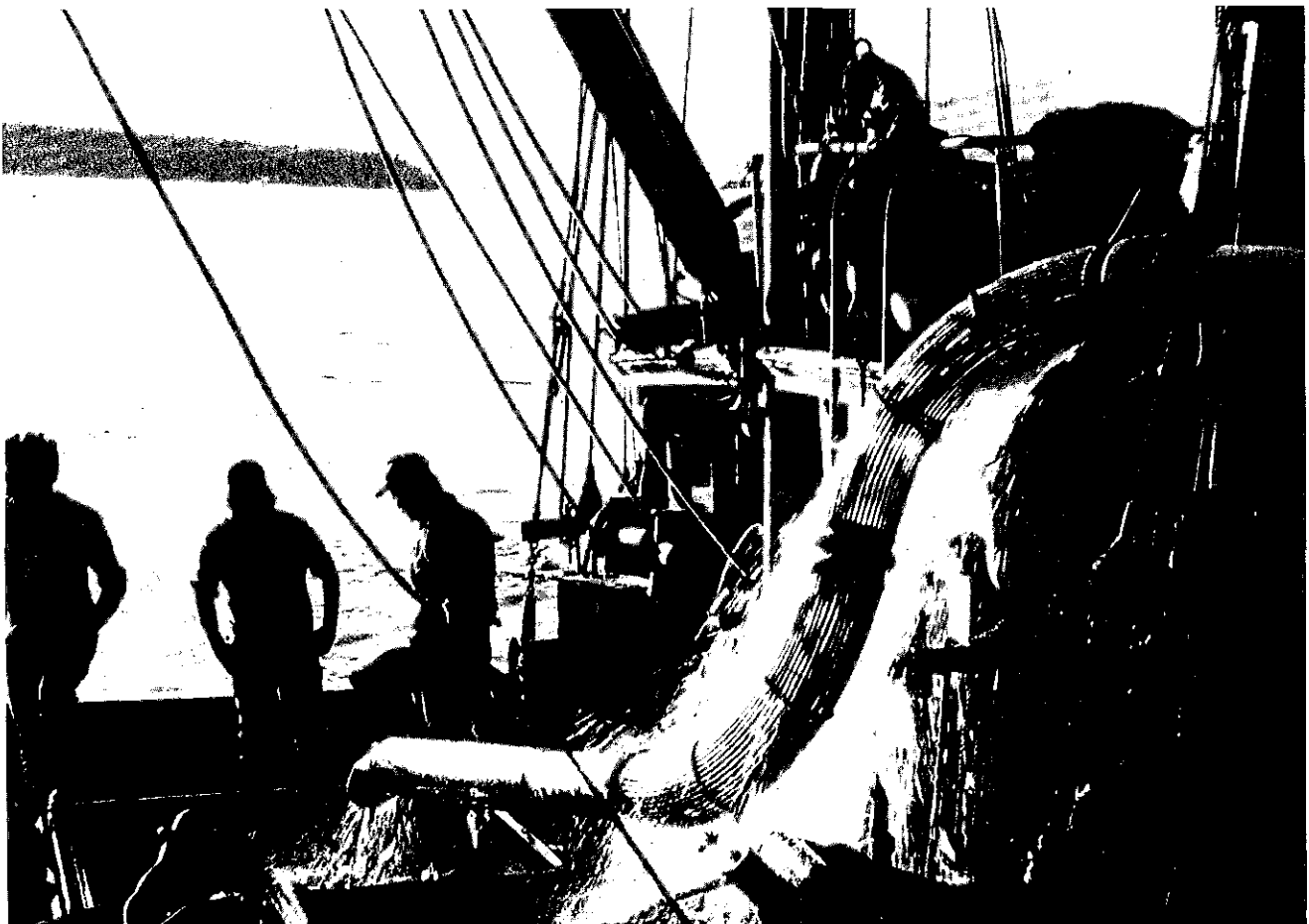
A herring pump and dewatering device are used to transfer roe herring from the net to the hold of a seine boat.
